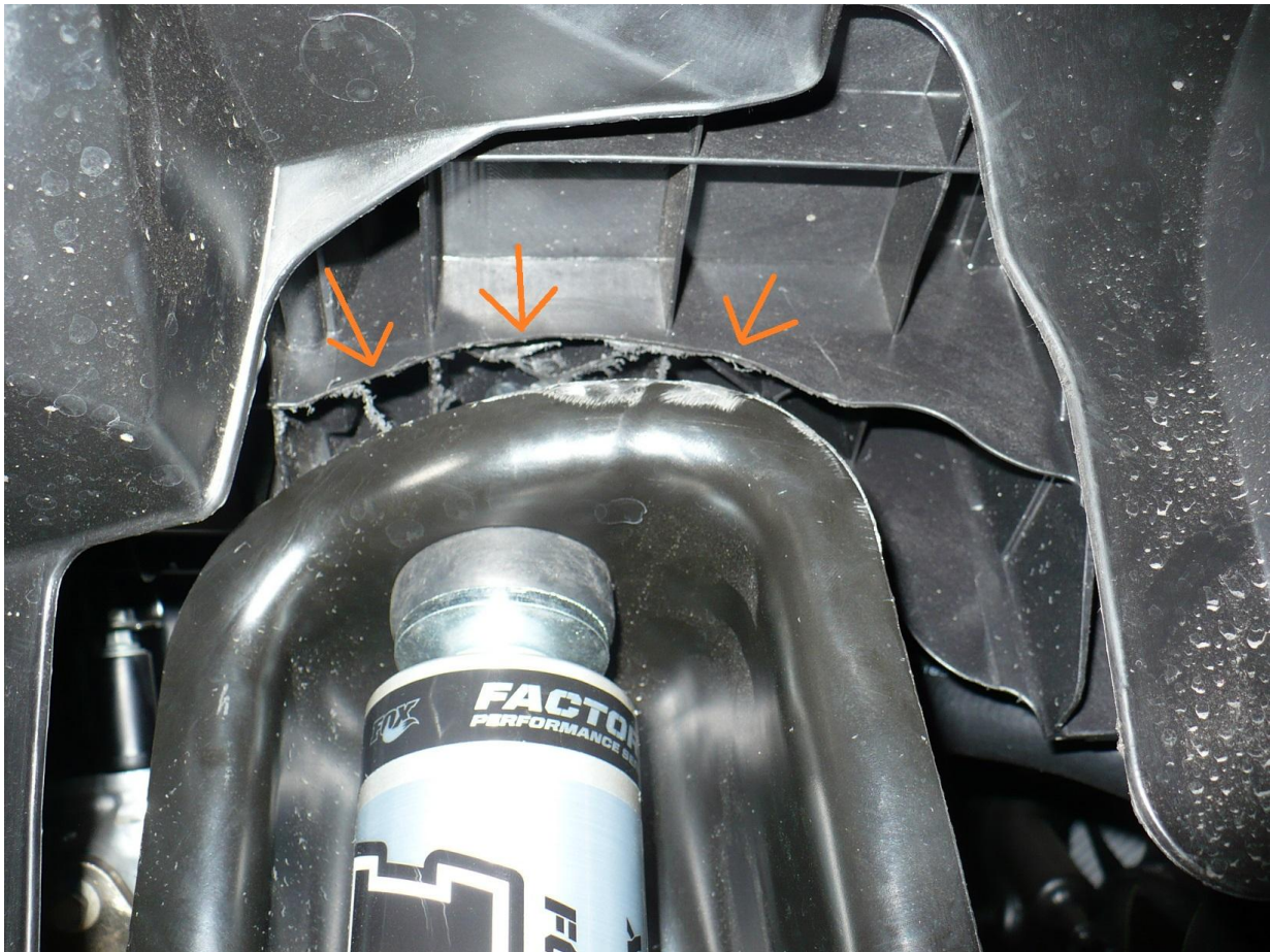
IMG 14.2 Red arrows indicate section to clearance for easier installation of upper shock nut.
