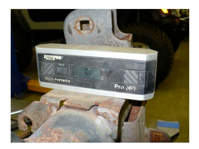
6. Measure the angle of the lower spring mount relative to the bumpstop pad, enter that angle here\_\_\_\_\_
