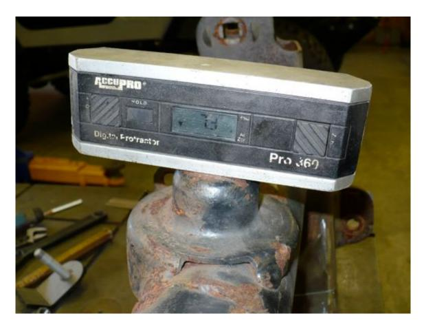
7. Take a reference measurement of the side to side position of the lower spring bracket.
