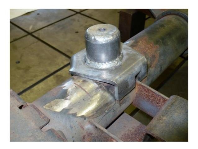
10. Rotate the spring mount forward to the desired angle from what it was originally, on a 4 dr JK, you typically want to rotate it about 10 degrees, a 2 dr JK is typically 15 degrees. You can also reference the upper spring mount and make the lower spring mount level to that. Just make sure the rear axle is at the correct ride height.
