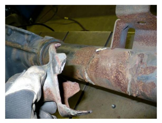
9. Position the new lower spring mounts on the axle tube, the same bracket is used on the left and right, the notch goes to the rear and is to clear the side of the rear track bar bracket, center the bracket side to side using the measurement for step 7.
