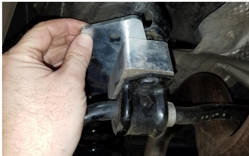
Figure 5. Sway Bar Spacer Plate Install on the Driver Side Sway Bar Mount
