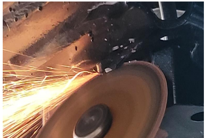
Figure 9. Cutting the Swaybar Drop spacer Welds
