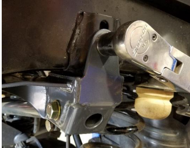
Figure 6. Torquing the 7/16" Thru Frame Bolt
