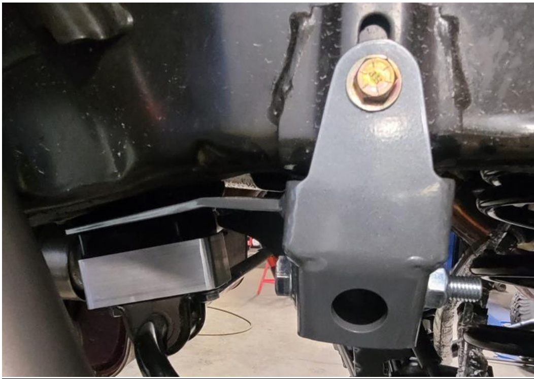
Figure 11. Track Bar Frame Brace Installed On 392 Wrangler
