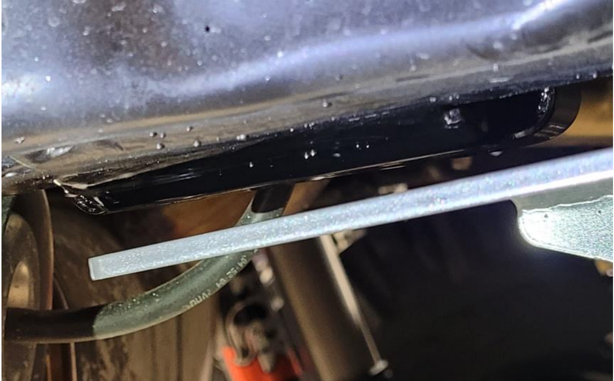
Figure 10. 1/4" Gap from Brace to Frame.
