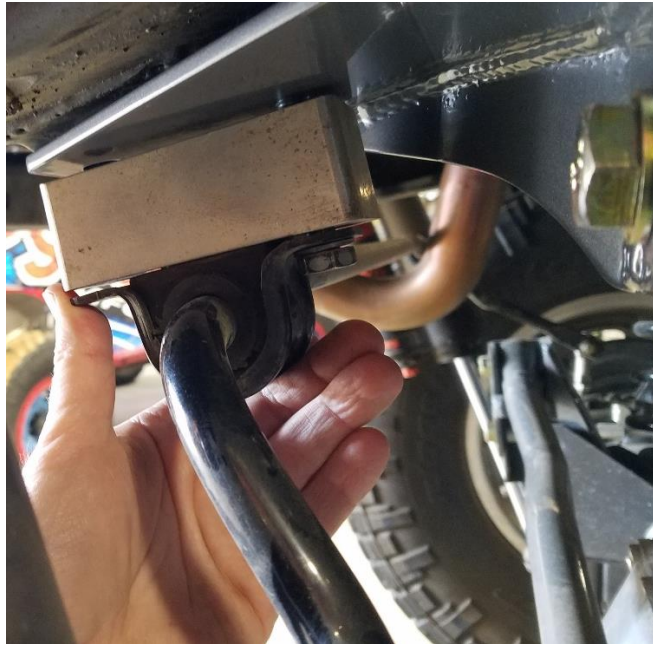
Figure 4. Installing the Passenger Side Rear Sway Bar Mount
