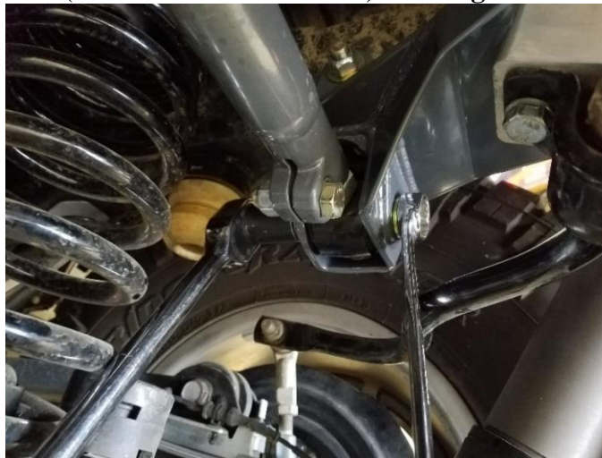
Figure 7. Torquing the Rear Track Bar Bolt
