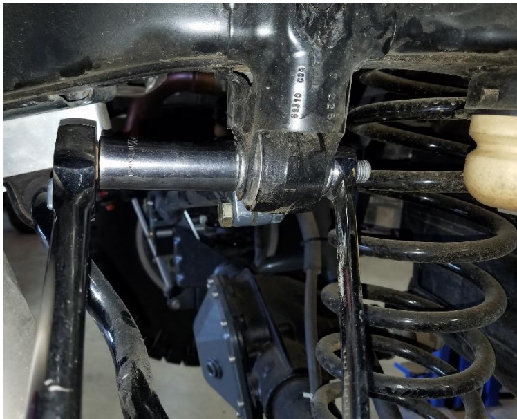
Figure 1. Removing Rear Track Bar from Mount
