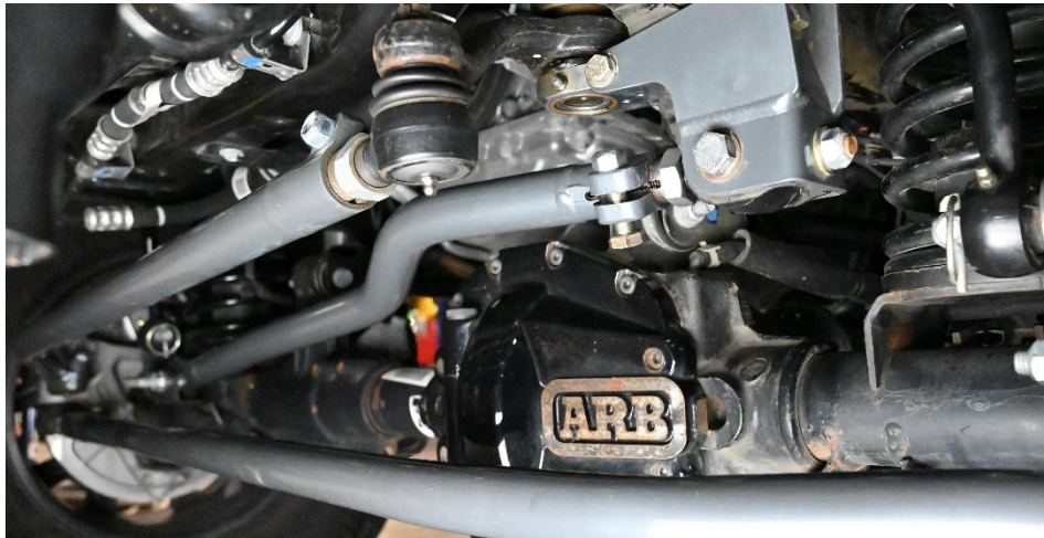
Figure 6. Correctly Installed Synergy Mfg Track Bar
