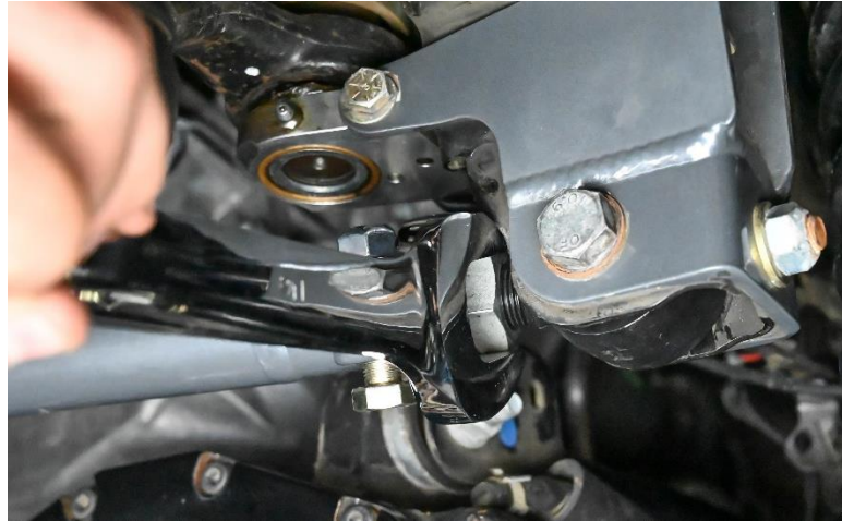
Figure 7. Adjusting the Track Bar to Center the Axle
