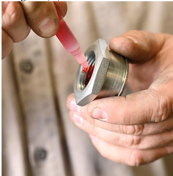
Figure 4. Adding Thread Locker to Nut
