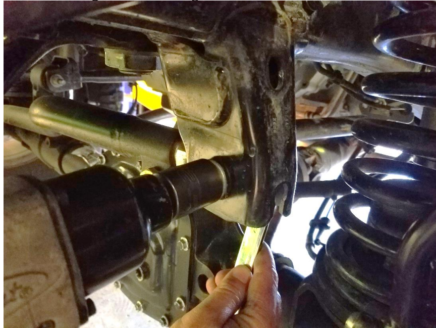
Figure 1. Removing Frame Side Track Bar Bolt
