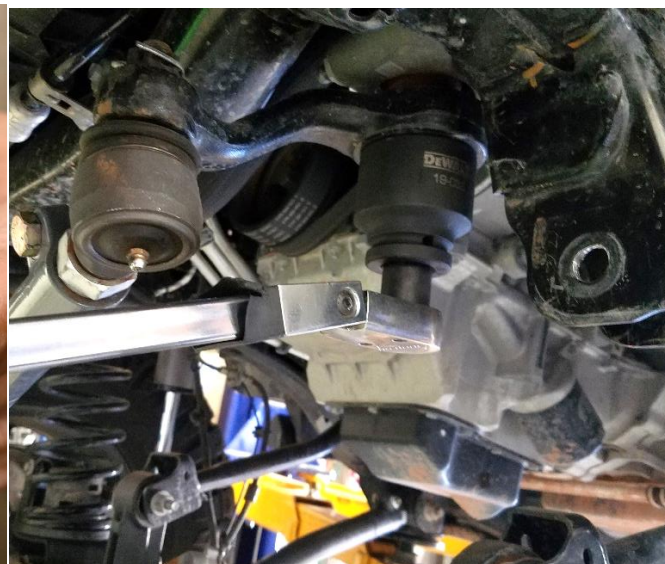
Figure 5. Torquing Pitman Arm Nut
