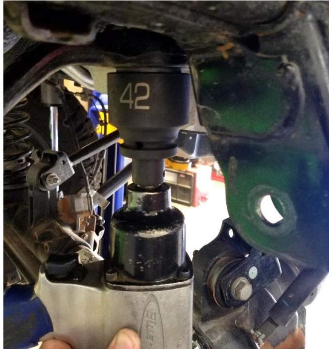
Figure 3. Removing Pitman Arm Nut.
