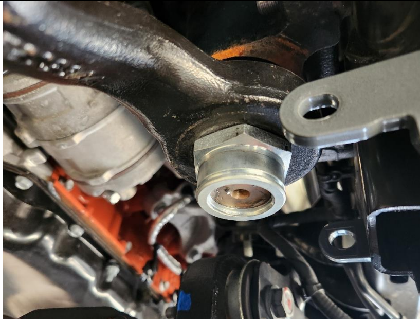
Figure 6. Pitman Arm Nut Installed
