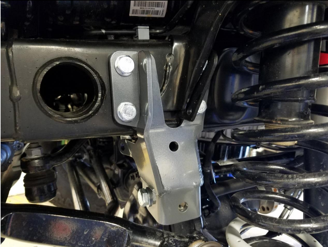
Figure 9. Threading Bolts into Steering Box
