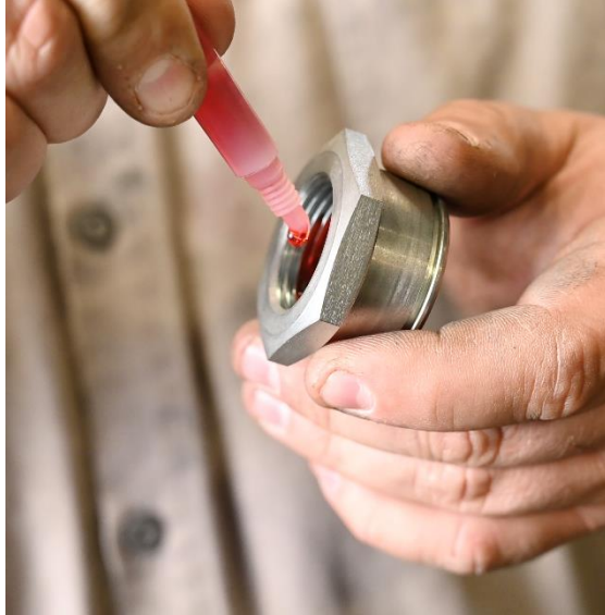
Figure 4. Adding Thread Locker to Nut
