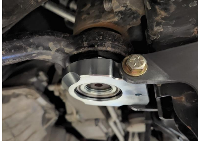
Figure 16. Installing Hardware in Synergy Sector Shaft Brace
