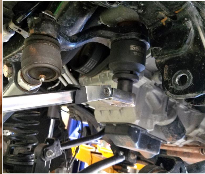
Figure 5. Torquing Pitman Arm Nut
