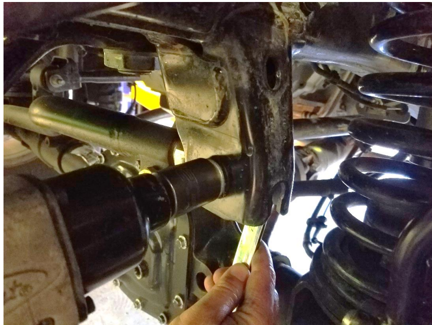
Figure 1. Removing Frame Side Track Bar Bolt
