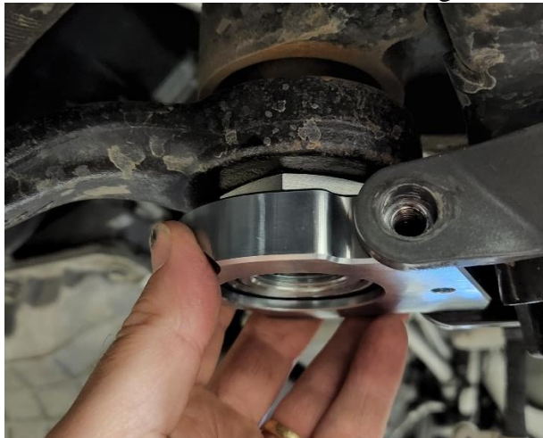
Figure 15. Installing Synergy Sealed Bearing Sector Shaft Brace
