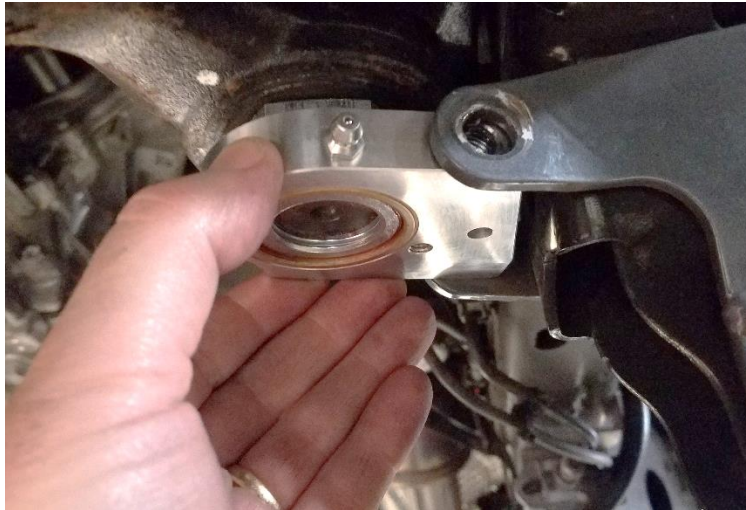
Figure 15. Installing Synergy Sector Shaft Brace on Pitman Arm Nut
