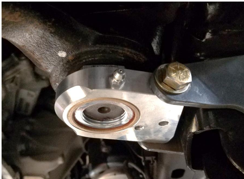
Figure 16. Installing Hardware in Synergy Sector Shaft Brace
