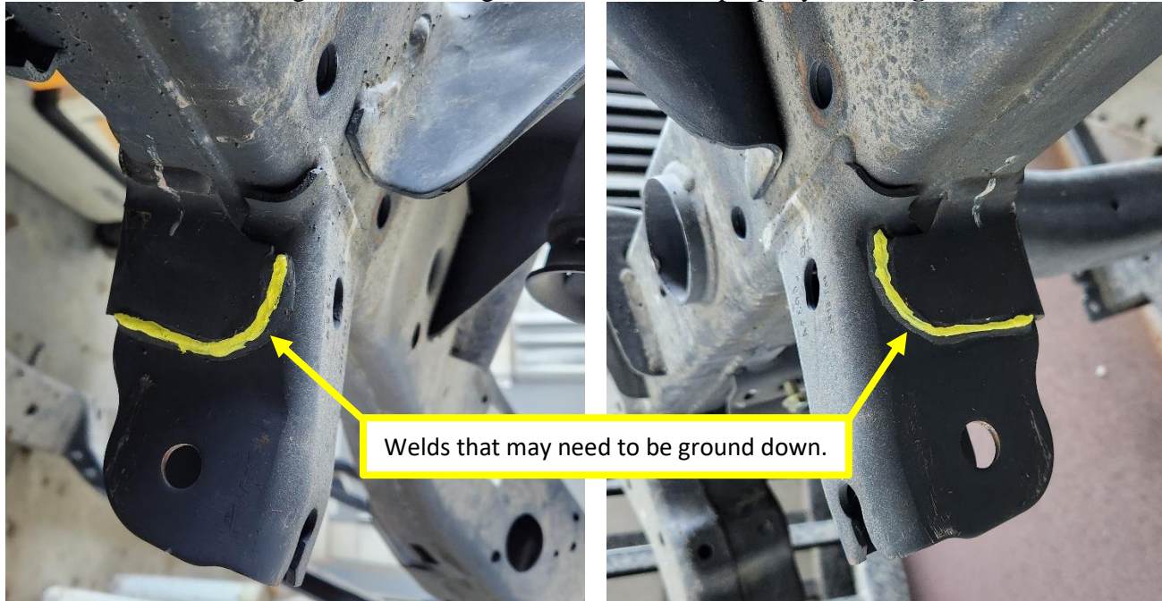
Figure 7. and 8. Track Bar Welds That May Need to be Ground Down.
