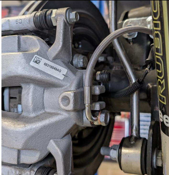
Figure 9. JL 392 Rear Caliper Banjo Bolt
