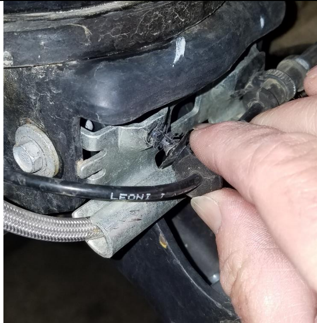
Figure 10. Reinstalling ABS Wiring Mounts.
