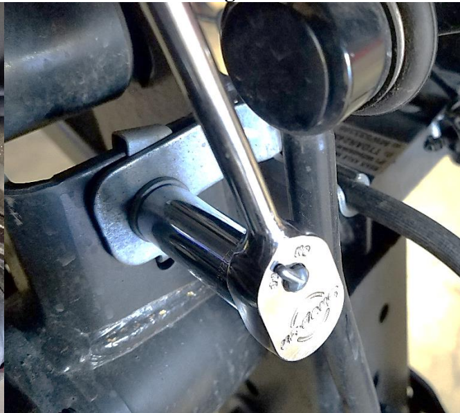
Figure 4. Rear Line Bracket Removal
