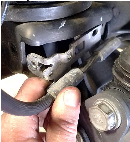
Figure 3. Front Line Bracket Removal
