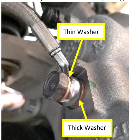
Figure 7. Front Caliper Banjo Bolt
