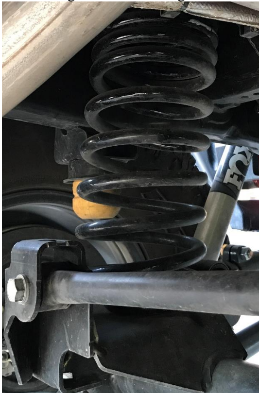
Figures 3 and 4. Correctly Installed Rear Springs
