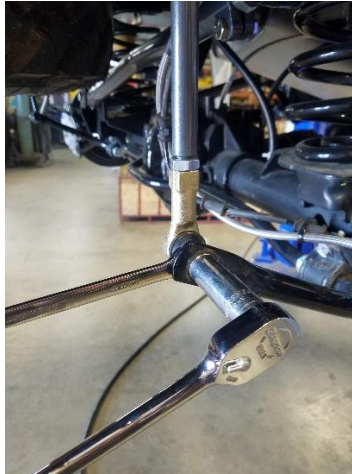
Figure 5. Tightening Lower Sway Bar TRE Stud and Nut.
