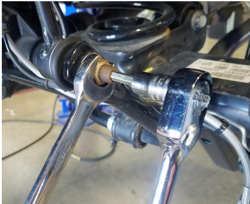
Figure 1. Loosening the Sway Bar Lower Tie Rod End.
