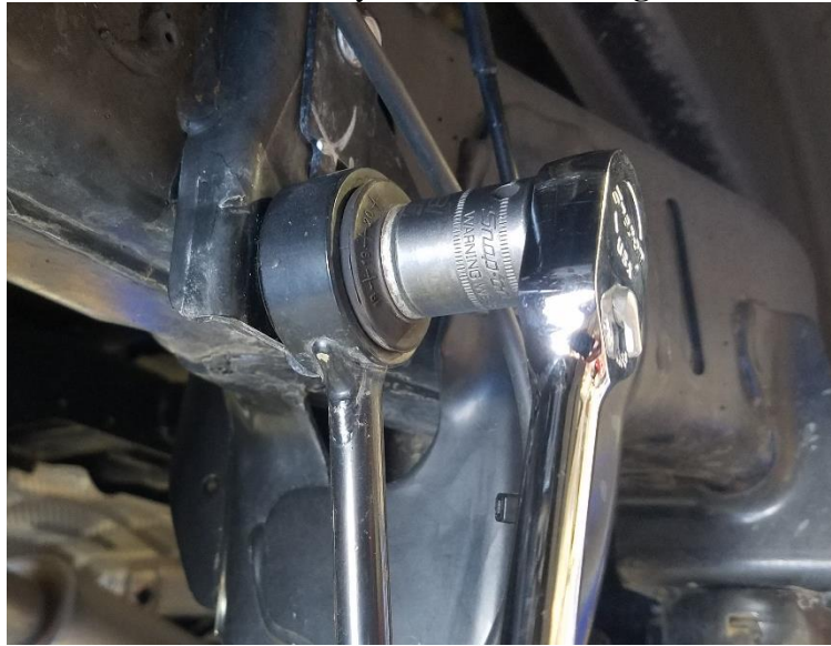
Figure 2. Removing the Upper Sway Bar Link Bolt on the Frame.
