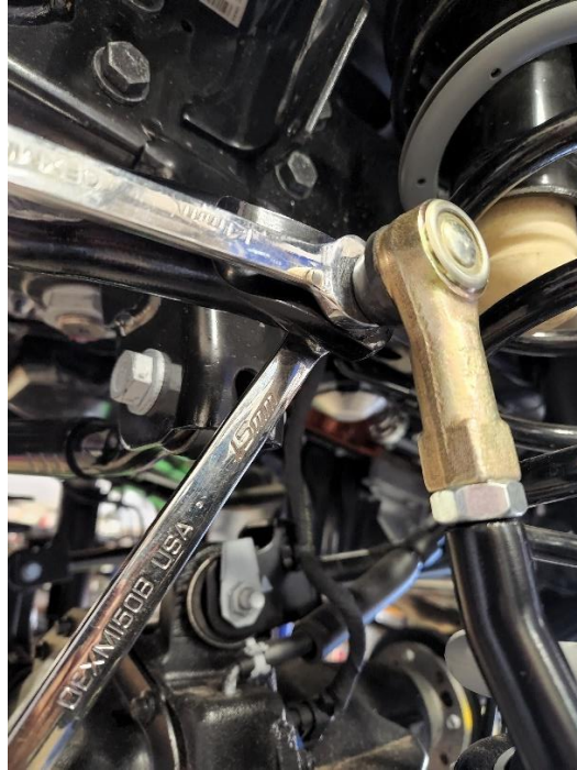
Figure 2. Installing the Driver's Side (Left) Sway Bar End Link
