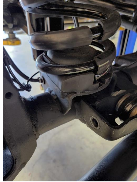
Figure 8. Tab Removed and Axle Cleaned Up.
