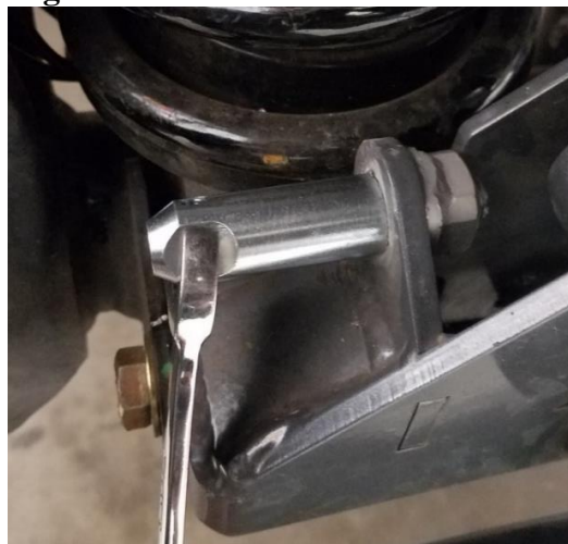
Figure 11. Passenger Side (Right) Disconnect Stud Installed with 8855-01 Front Track Bar Relocation Bracket
