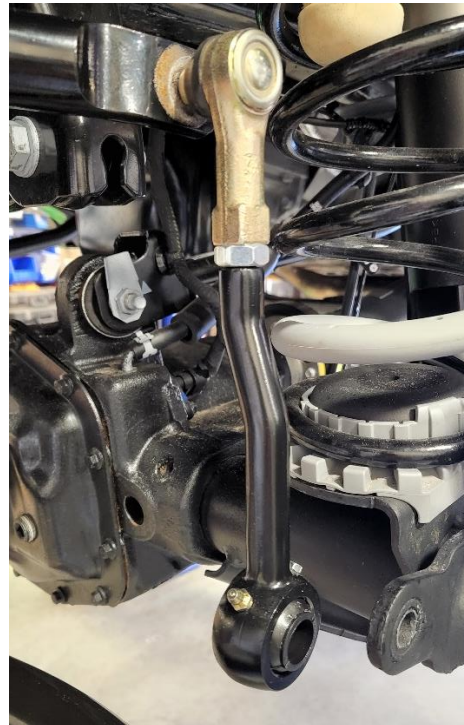
Figure 3. Correctly Oriented Driver's Side (Left) Sway Bar End Link
