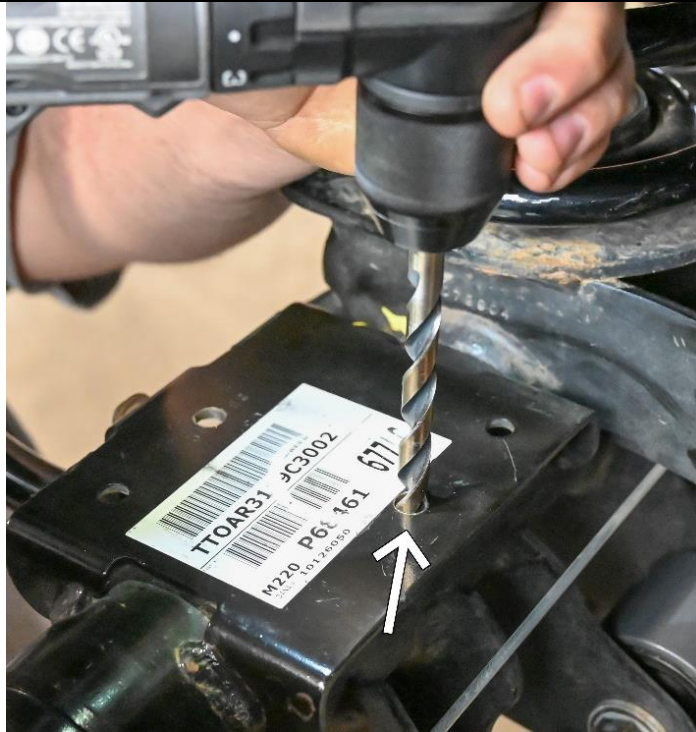
Figure 5. Drilling the Mounting Holes in the Bumpstop Pad.
