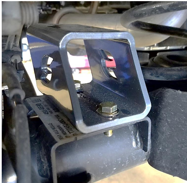
Figure 1. Lining up Bolt Holes and Inserting Bolts.
