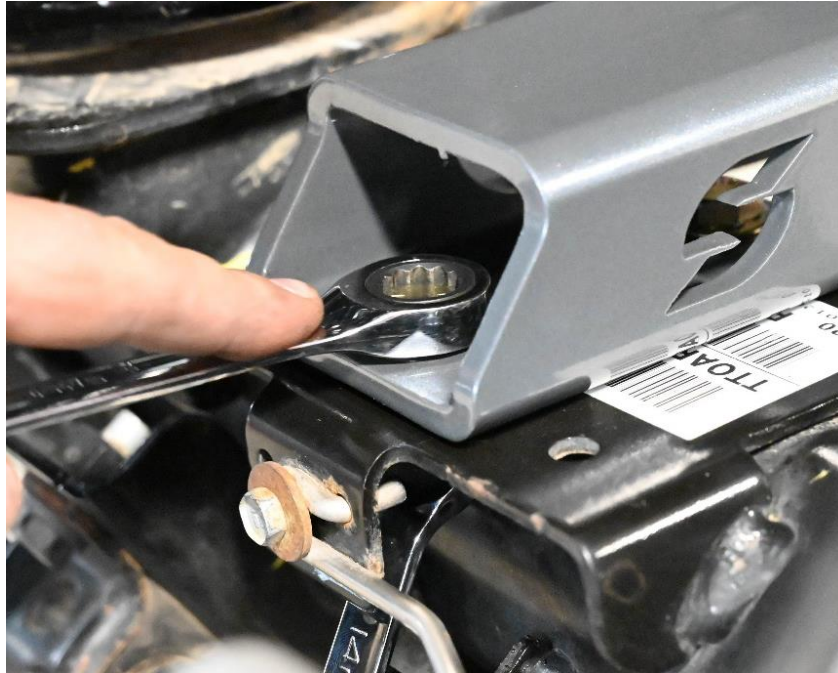
Figure 7. Tightening the Two 3/8-16 Bolts and Nuts.
