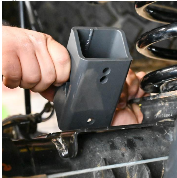
Figure 6. Installing the Bumpstop Extension
