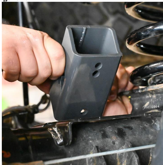
Figure 7. Installing the Bumpstop Extension
