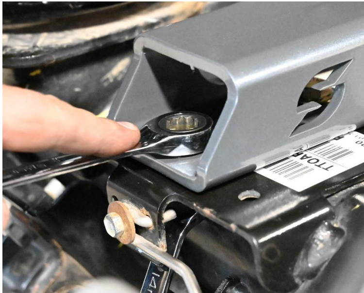
Figure 8. Tightening the Two 3/8-16 Bolts and Nuts.
