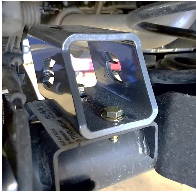
Figure 1. Lining up Bolt Holes and Inserting Bolts.
