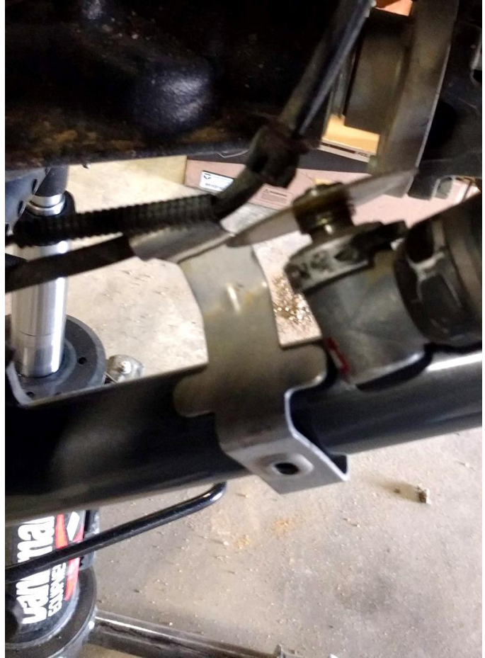
Figures 1 and 2. Marking and Trimming Factory Brake Line Bracket
