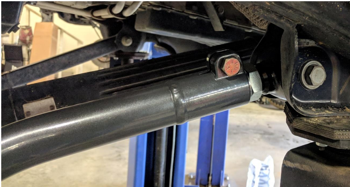
Figure 4. Control Arm Correctly Installed (Frame Side Shown)
