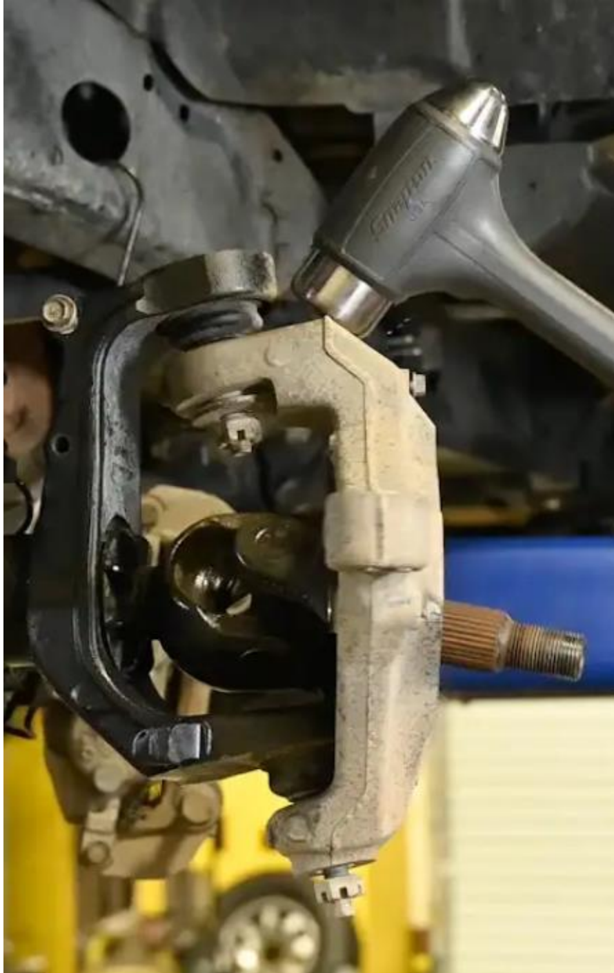
Figure 7. Separating the Upper Ball Joint
