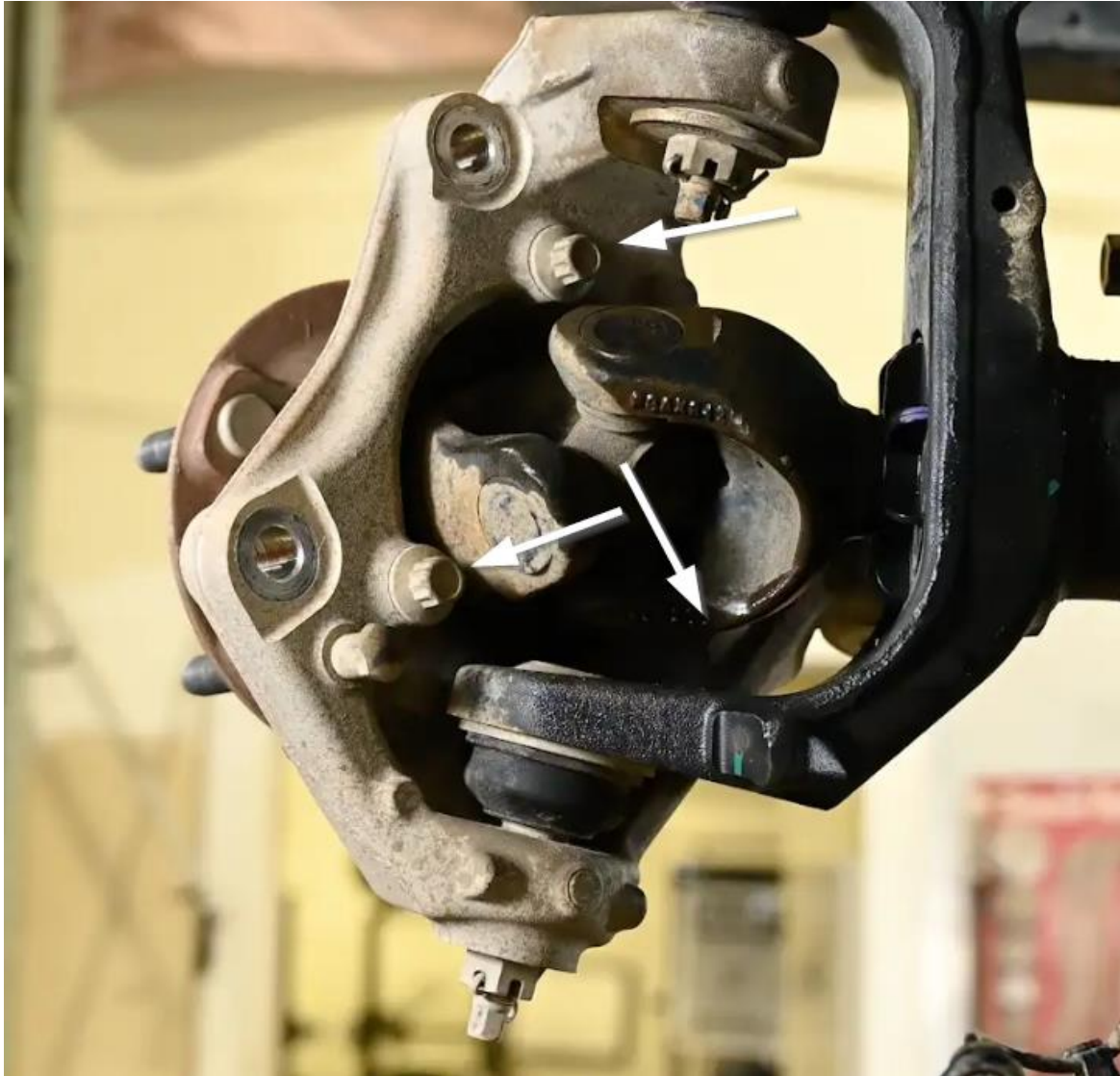
Figure 5. Unit Bearing Retention Bolts
