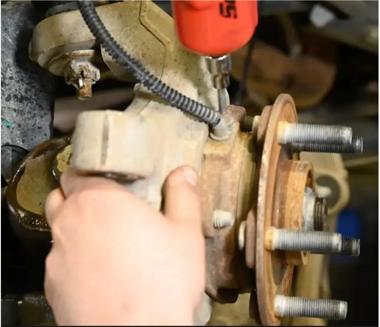
Figure 4. Wheel Speed Sensor
