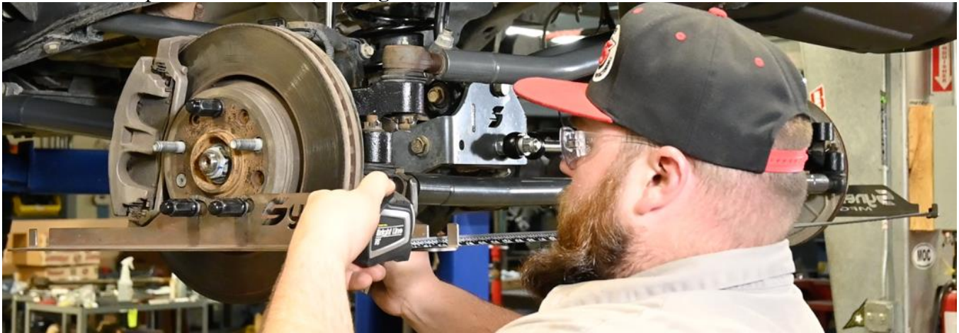
Figure 10. Adjusting Toe with Synergy Alignment Plates
