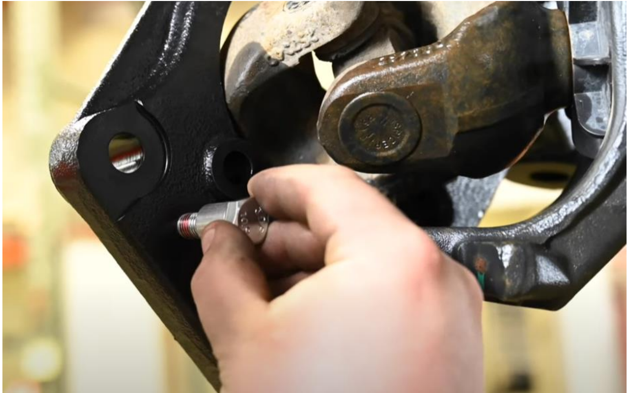
Figure 9. Steering Stop Spacer Being Installed
