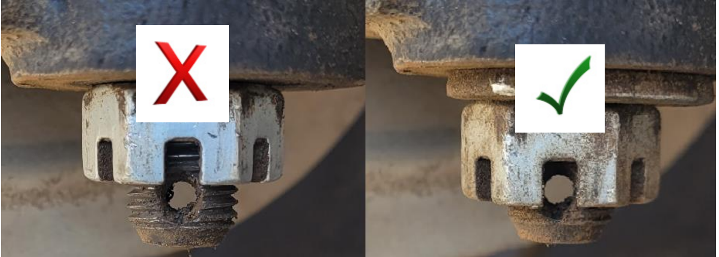
Figure 8. Cotter Pin Alignment on Lower Ball Joint
