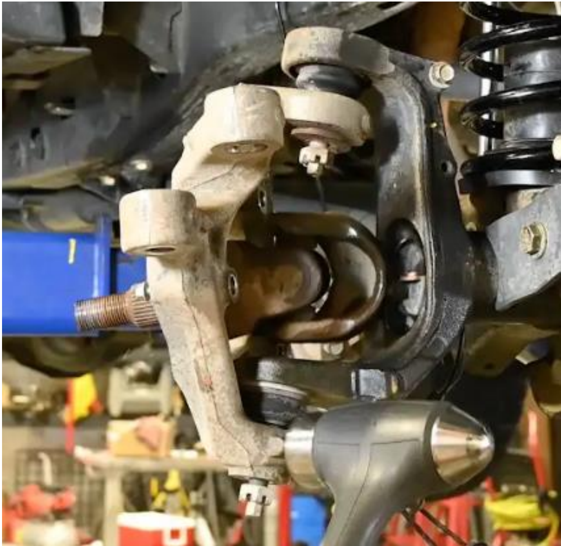
Figure 6. Separating the Lower Ball Joint
