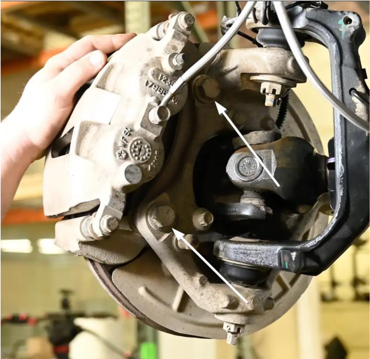
Figure 2. Caliper Adapter bolts
