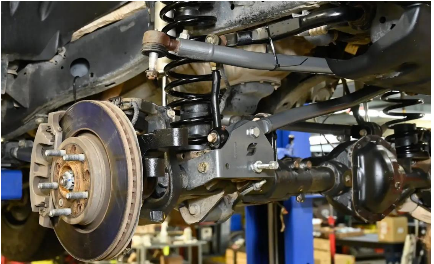
Figure 1. Steering Removed and Drag Link Hung Out of the Way
