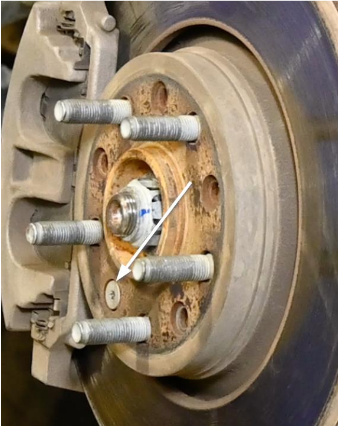
Figure 3. Rotor Retention Bolt
