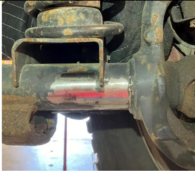
Figure 11. Driver Side Sway Bar Tab Removed from the Axle Tube
