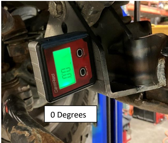
Figures 21 and 22. Angle Finder Zeroed on the Front Face of the Track Bar Bracket and the New Sway Bar Tab Set at 70 Degrees on the Axle Tube.
