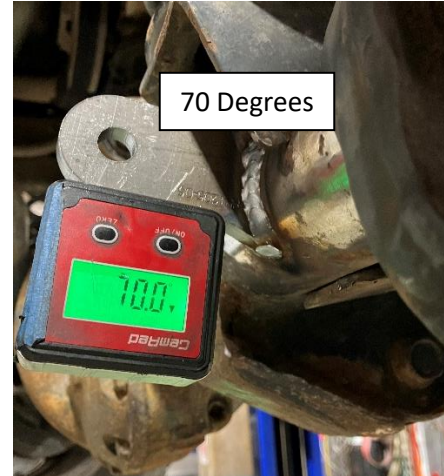
Figures 21 and 22. Angle Finder Zeroed on the Front Face of the Track Bar Bracket and the New Sway Bar Tab Set at 70 Degrees on the Axle Tube.
