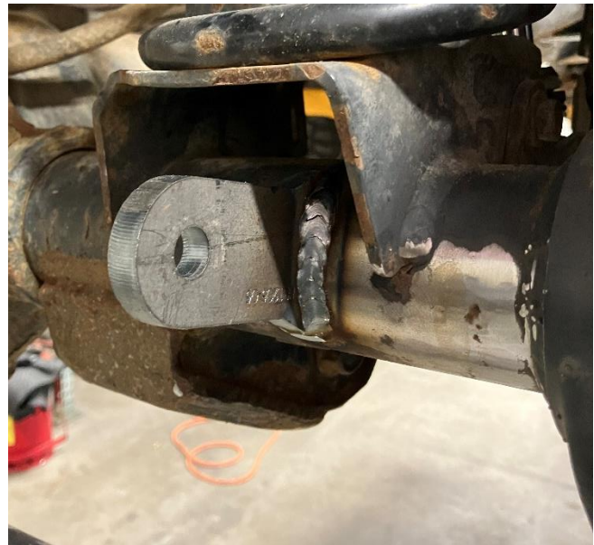
Figures 23 and 24. Fully Welded Sway Bar Tab on the Driver Side Axle Tube
