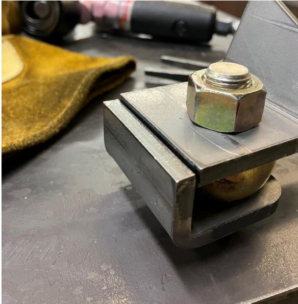
Figure 25. Hydro Tabs Bolted to 5/8" Rod End
