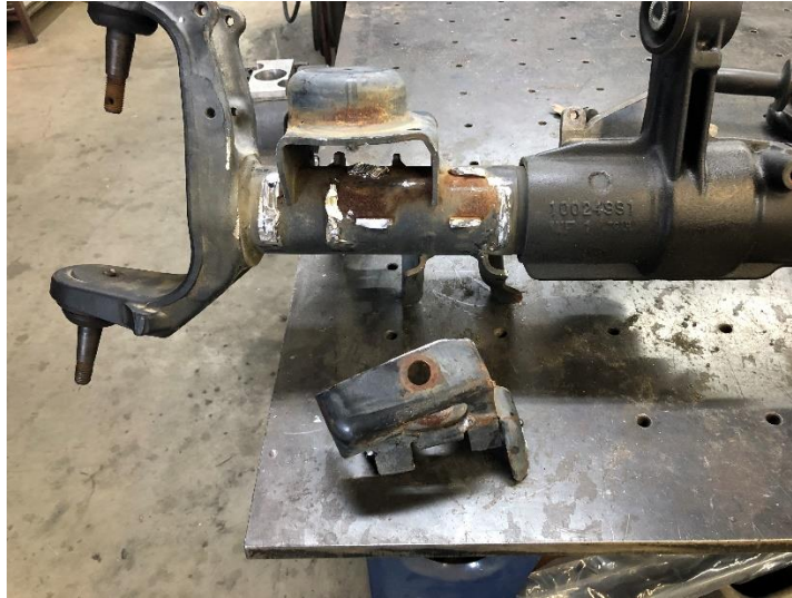
Figure 2. Removed Factory Track Bar Bracket
