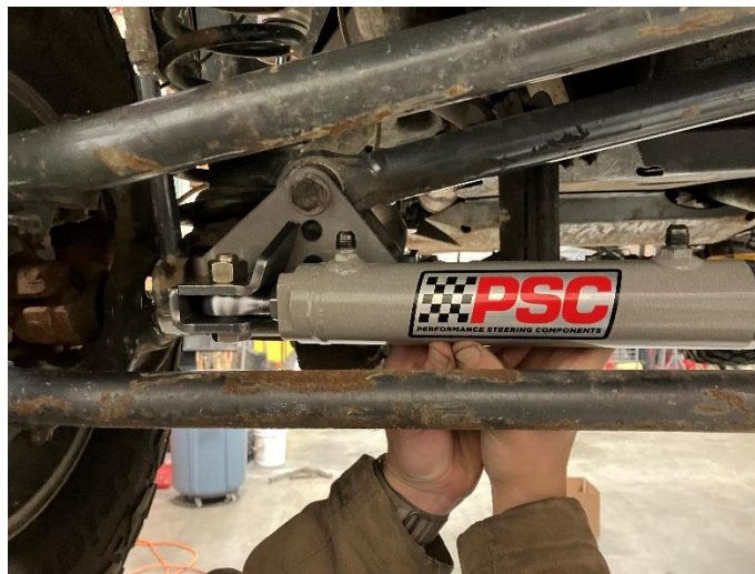
Figure 27. Hydro Assist Ram and Weld Tabs Placed on the Track Bar Bracket
