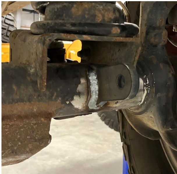
Figures 23 and 24. Fully Welded Sway Bar Tab on the Driver Side Axle Tube
