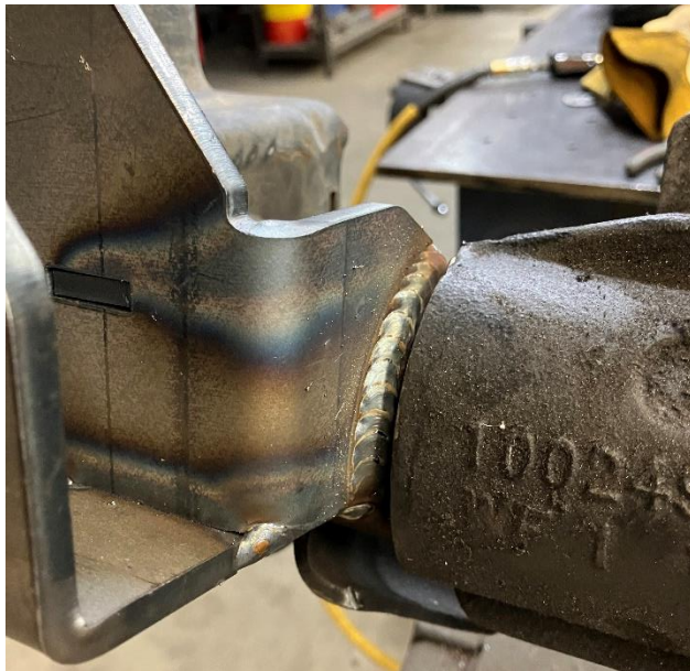
Figure 9. Vertical Weld Against FAD
