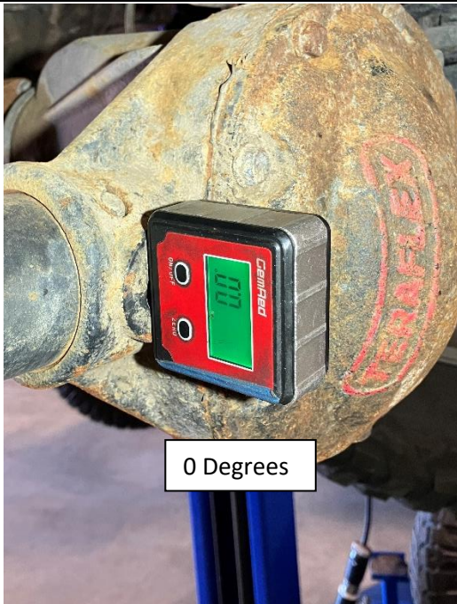
Figures 13 and 14. Front Face of Track Bar Bracket Parallel to the Spreader Holes on the Differential
