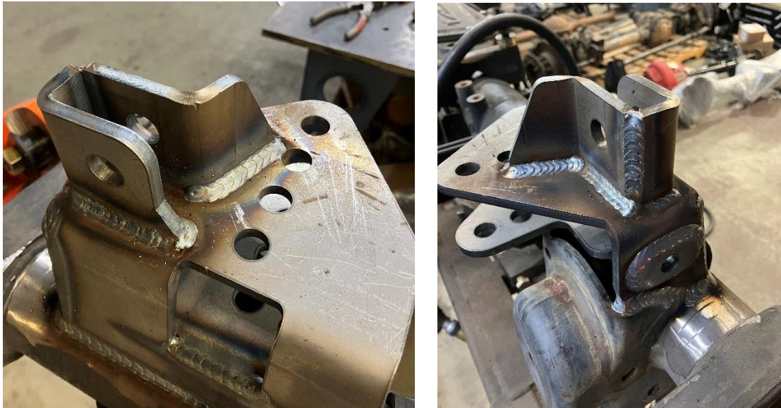
Figures 28 and 29. Hydro Mount Fully Welded on the Track Bar Bracket
