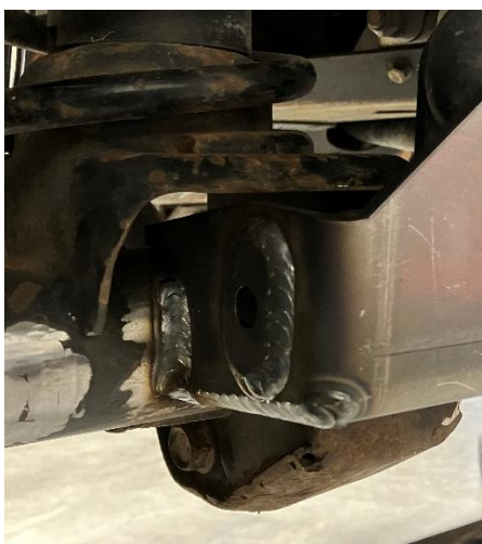
Figures 15 and 16. Completed Vertical Welds on Either Side of the Track Bar Bracket.
