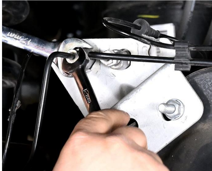
Figure 2. Disconnecting Brake Lines.
