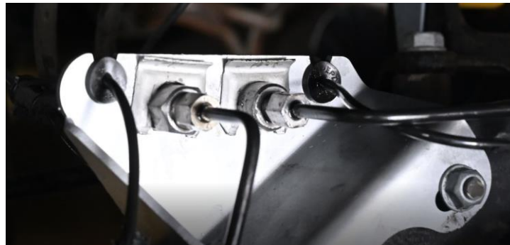
Figure 5. Reinstalled Brake Line Clips and ABS Wires.
