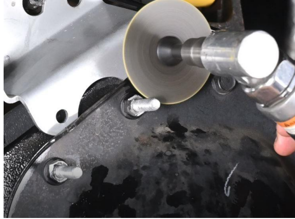
Figure 4. Cutting Down Brake Line Bracket Mounting Stud.
