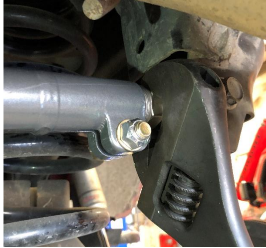
Figure 4. Adjusting the Rear Track Bar to Align the Axle Side Bolt.
