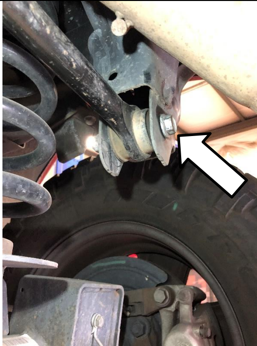
Figure 2. Bolt to Remove the Track Bar from the Frame Side.
