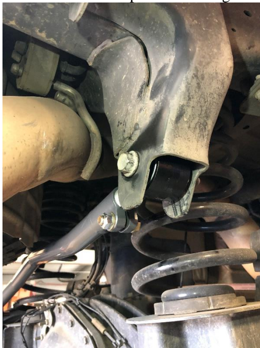
Figure 3. Installing the Synergy Mfg Track Bar at the Frame.
