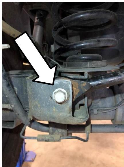
Figure 1. Bolt to Remove the Track Bar from the Axle Side.
