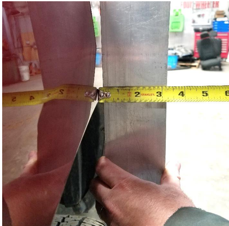
Figure 5. Measuring the Distance from the Tire Face to the Fender.
