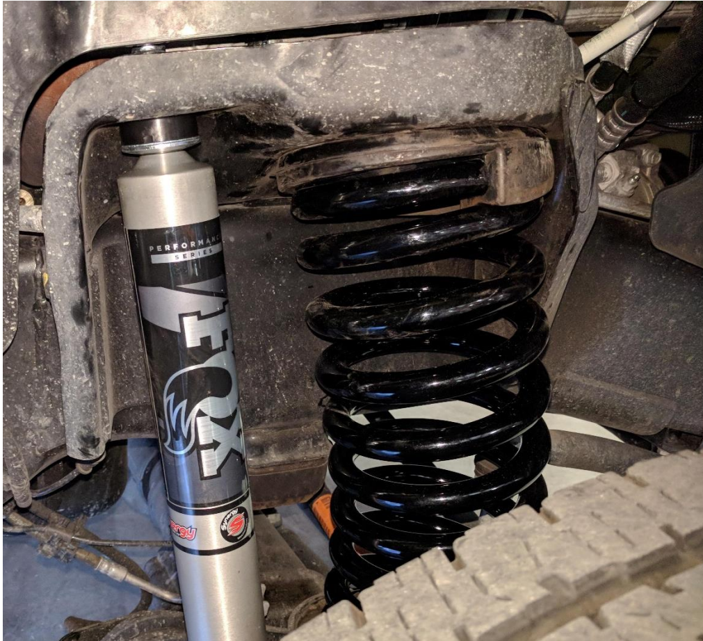
Figure 4. Front Shocks and Springs Correctly Installed
