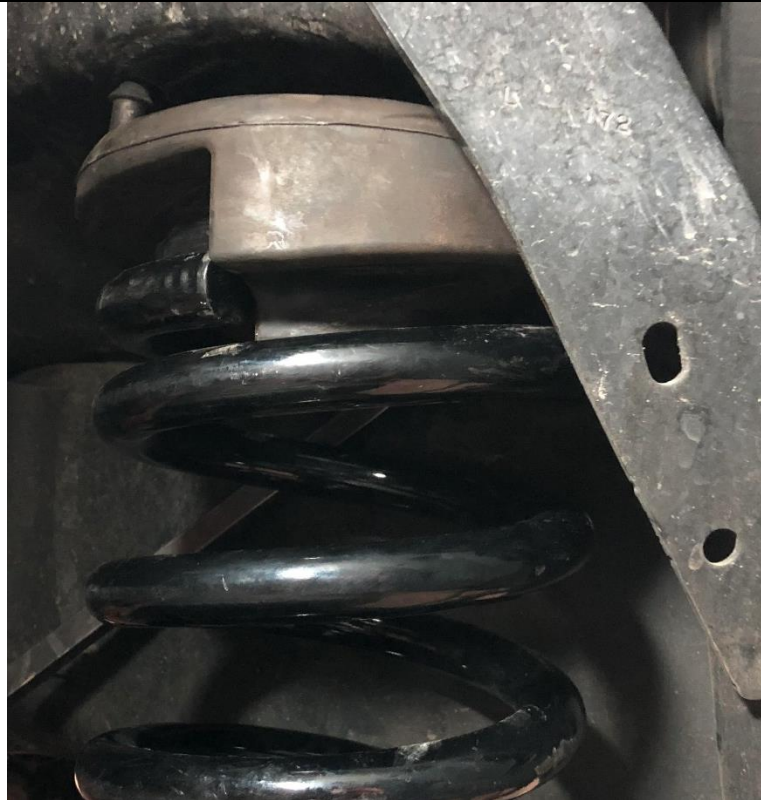
Figure 2. Synergy Leveling Spring Installed, Spring Isolator Not Fully Seated
