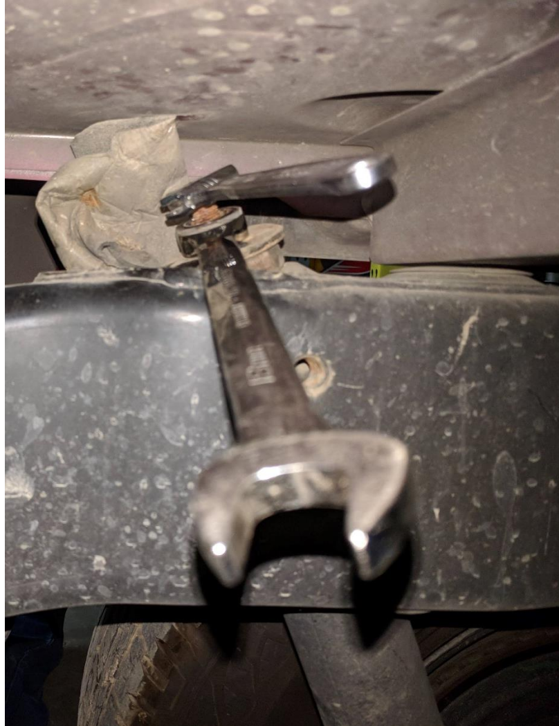
Figure 5. Using Two Wrenches to Remove Rear Shock Upper Nut
