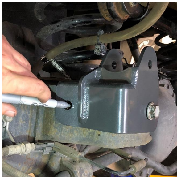
Figure 6. Marking the Factory Bracket for Drilling.
