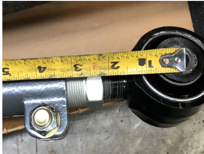
Figure 12. Max Distance from the End of the Bar to the Bushing Center.
