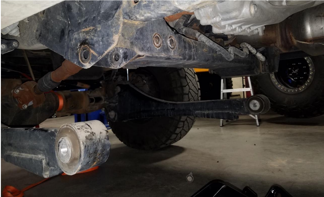
Figure 3. Radius Arms Separated from Frame
