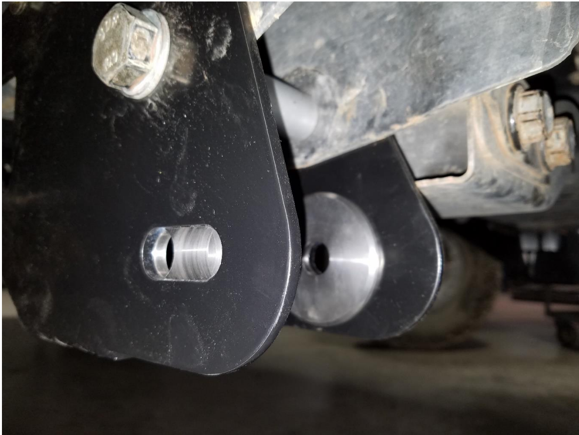
Figure 10. Radius Arm Position Spacers Installed
