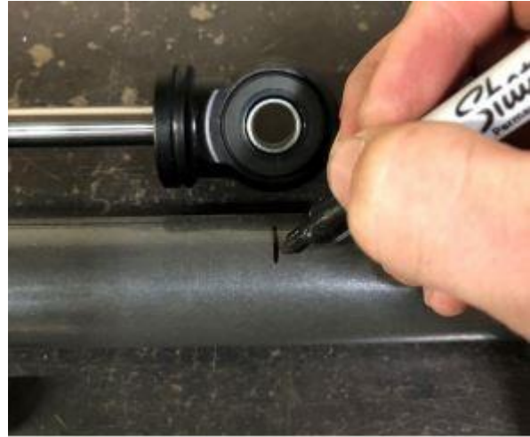
Figure 7. Marking the Mount Centerline
