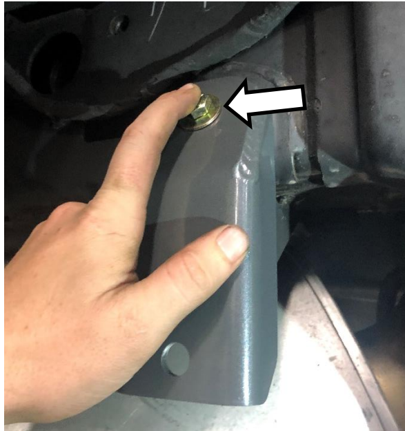
Figure 2. Installing 8708 bracket with 3/8 bolt.
