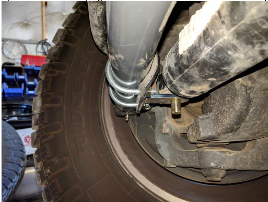
Figure 5. Clamp Installed with Bolt Perpendicular to Ground
