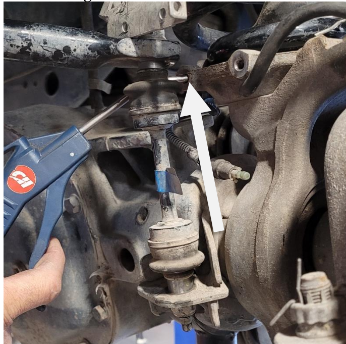
Figure 2. Cleaning the Inner Hole
