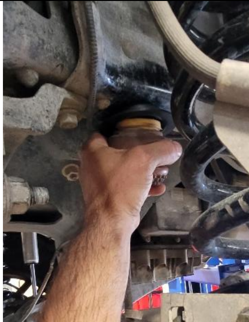
Figure 14. Removing the Factory Bump Stop
