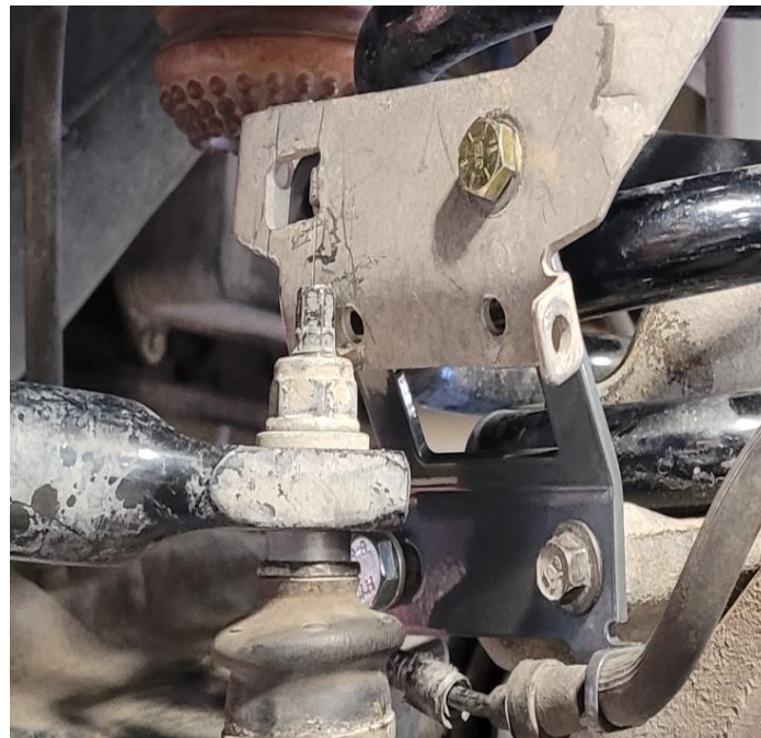
Figure 12. Correct Orientation of Driver Side Bracket
