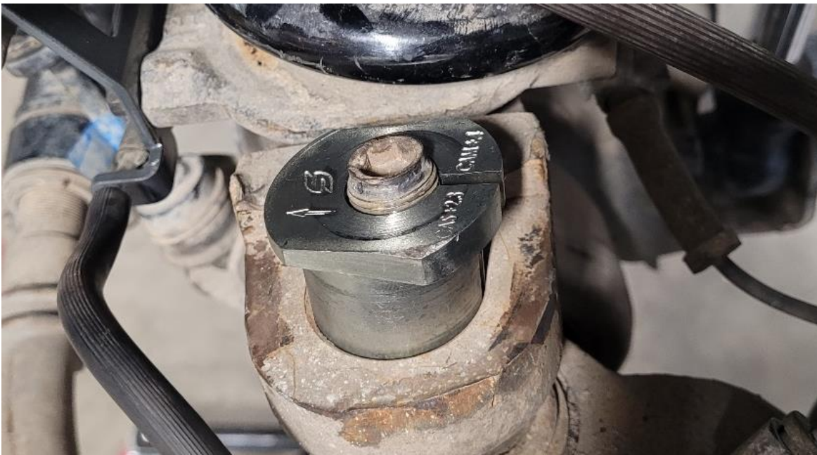
Figure 22. Start the Sleeve With the Arrow Pointing Toward the Front of the Vehicle
