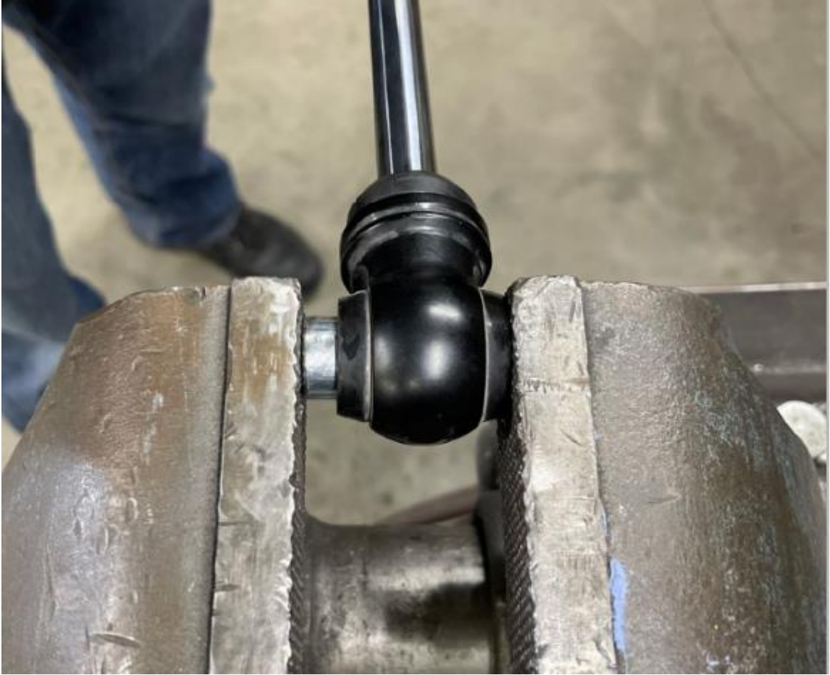
Figure 27: Finishing New Bushing Installation
