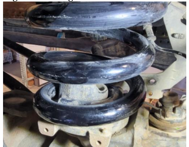
Figure 8. Passengers Side Lower Spring Orientation
