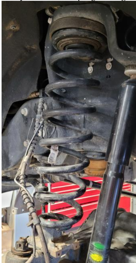
Figure 5. Spring Ready for Removal
