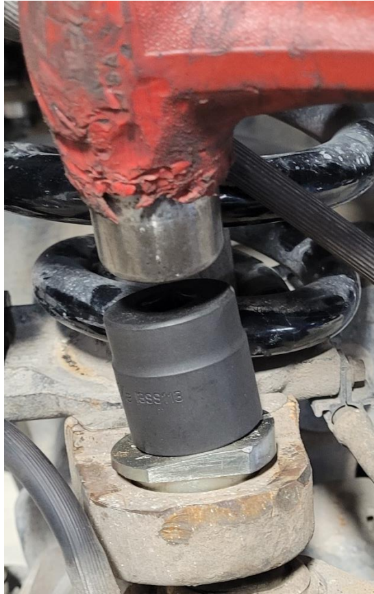
Figure 23. Tapping the Sleeve Into Position
