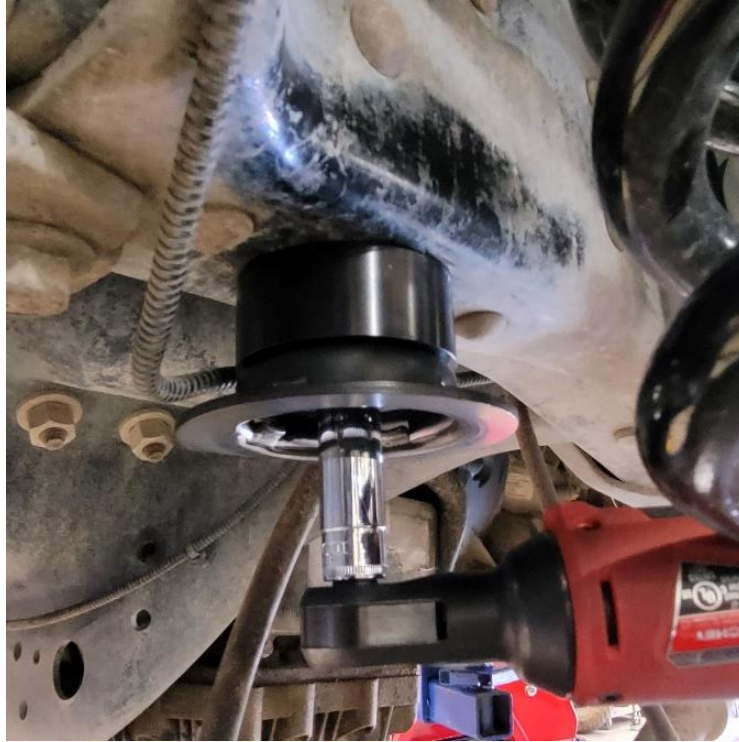
Figure 18. Installing the Spacer and Cup
