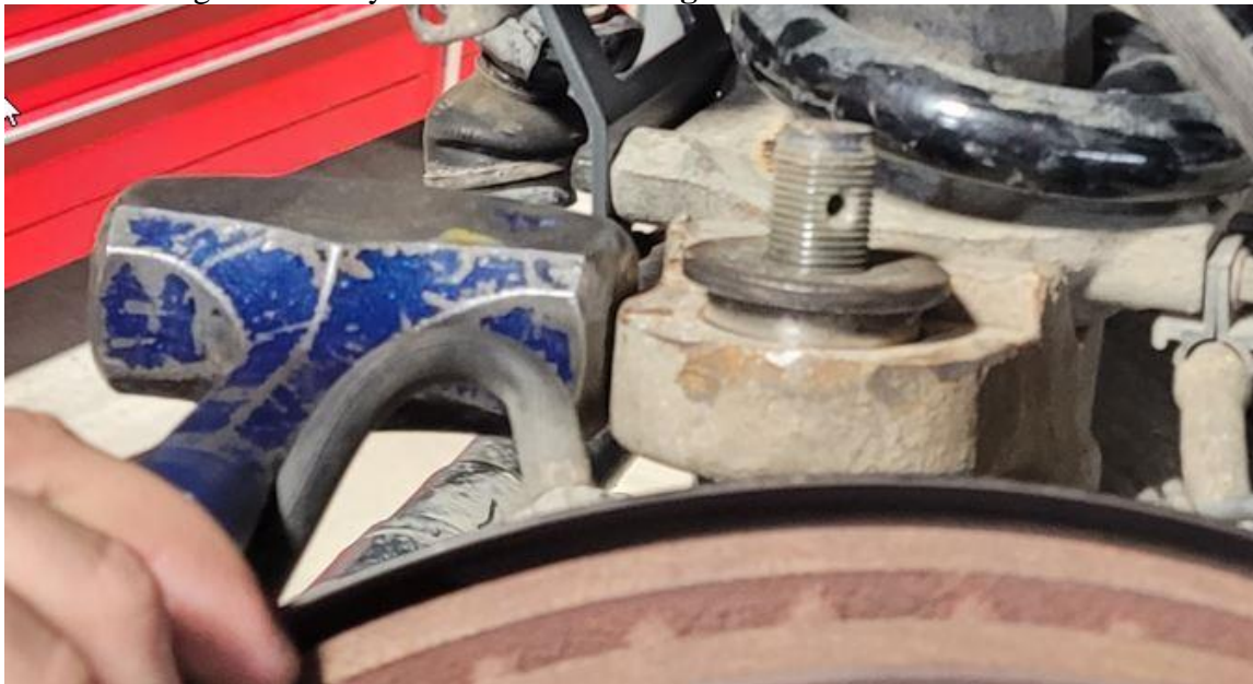
Figure 20. Dislodging the Factory Caster Sleeve
