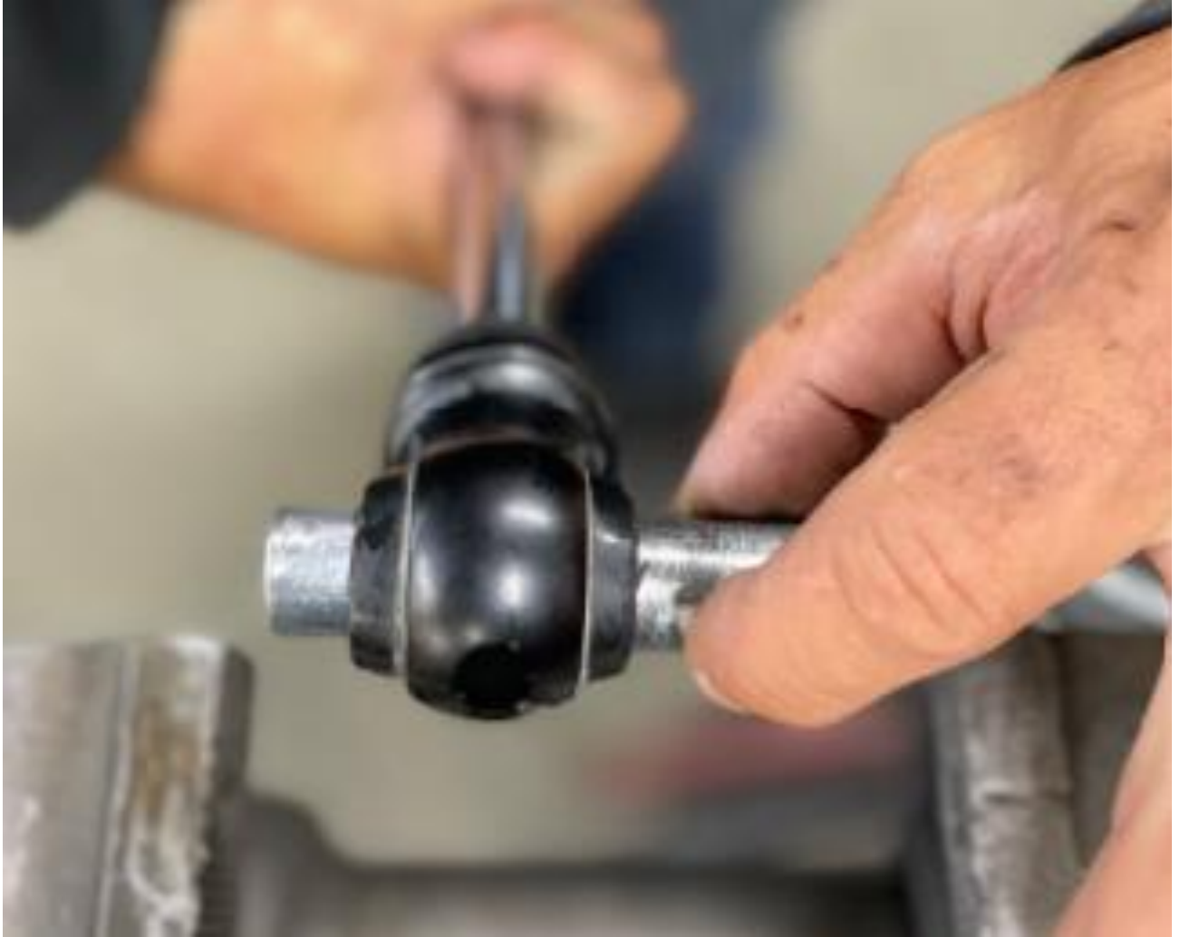
Figure 26: Wiggling Out the Old Eyelet Sleeve
