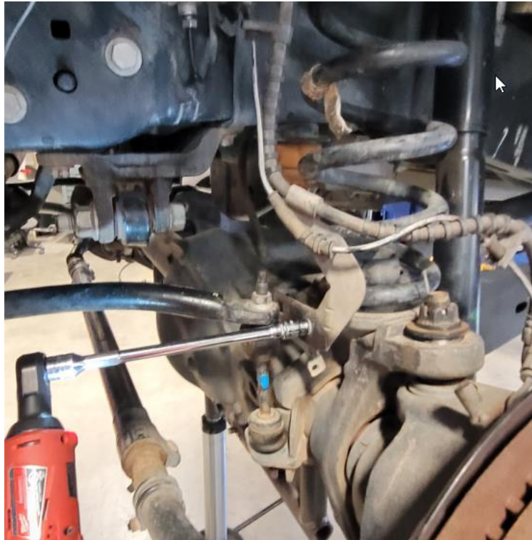
Figure 2. Brake Line Bracket Removal
