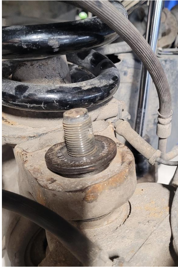
Figure 19. Drivers Side Nut and Cotter Pin Removed from Upper Ball Joint
