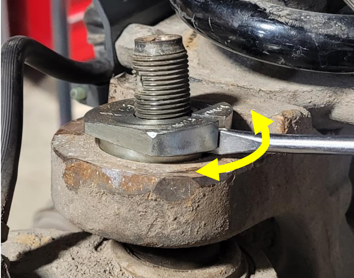
Figure 24. Rotating the Sleeve with a Screw Driver to Fine Tune Camber
