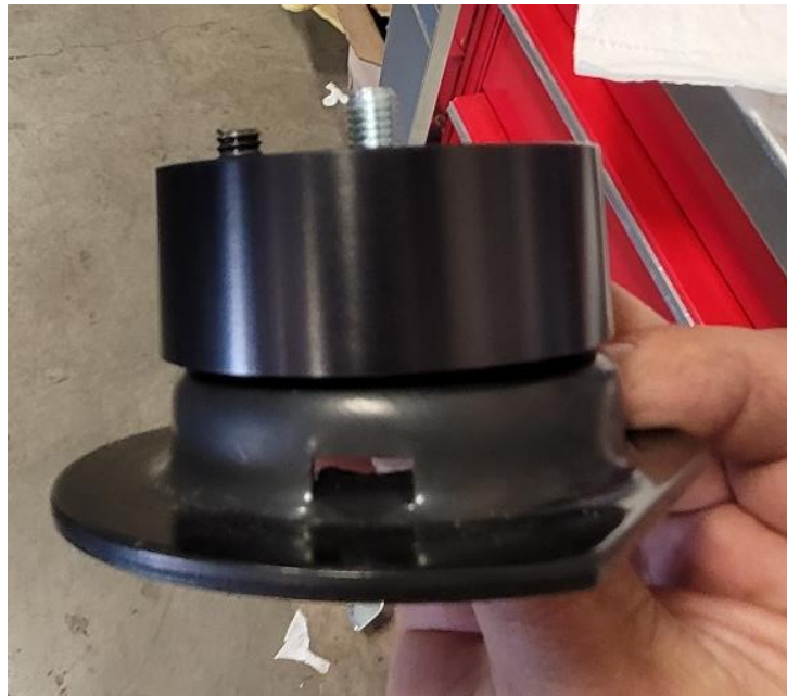
Figure 17. Spacer and Cup Aligned for Installation
