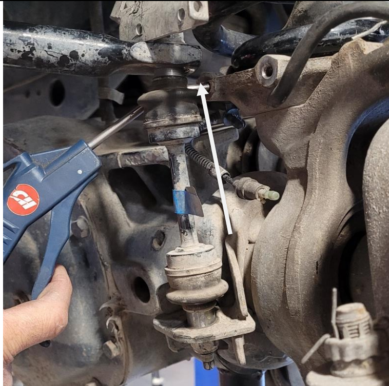
Figure 11. Cleaning the Inner Hole
