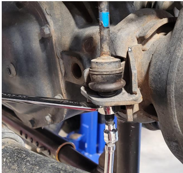
Figure 3. Removing the Lower Sway Bar End Link Nut
