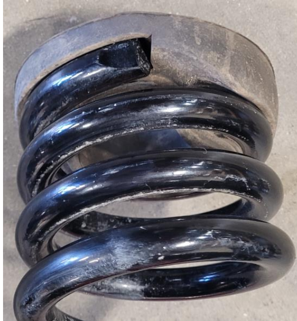
Figure 6. Isolator Pad Correctly Positioned on the Top of the Spring
