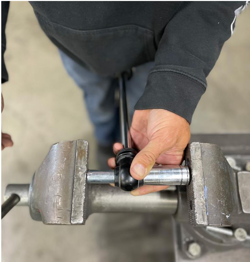
Figure 25. Shock Eyelet Setup in the Vice
