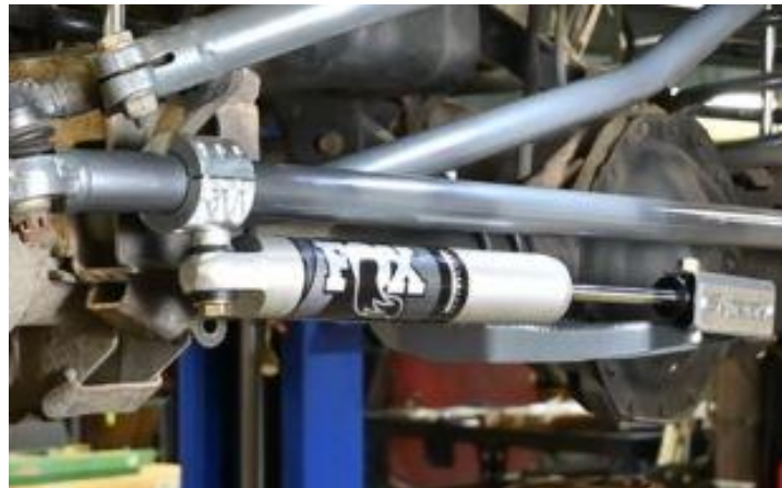
Figure 6. Correctly Installed Stabilizer
