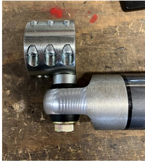
Figure 5. 4050-75 Clamp Installed on Steering Stabilizer.
