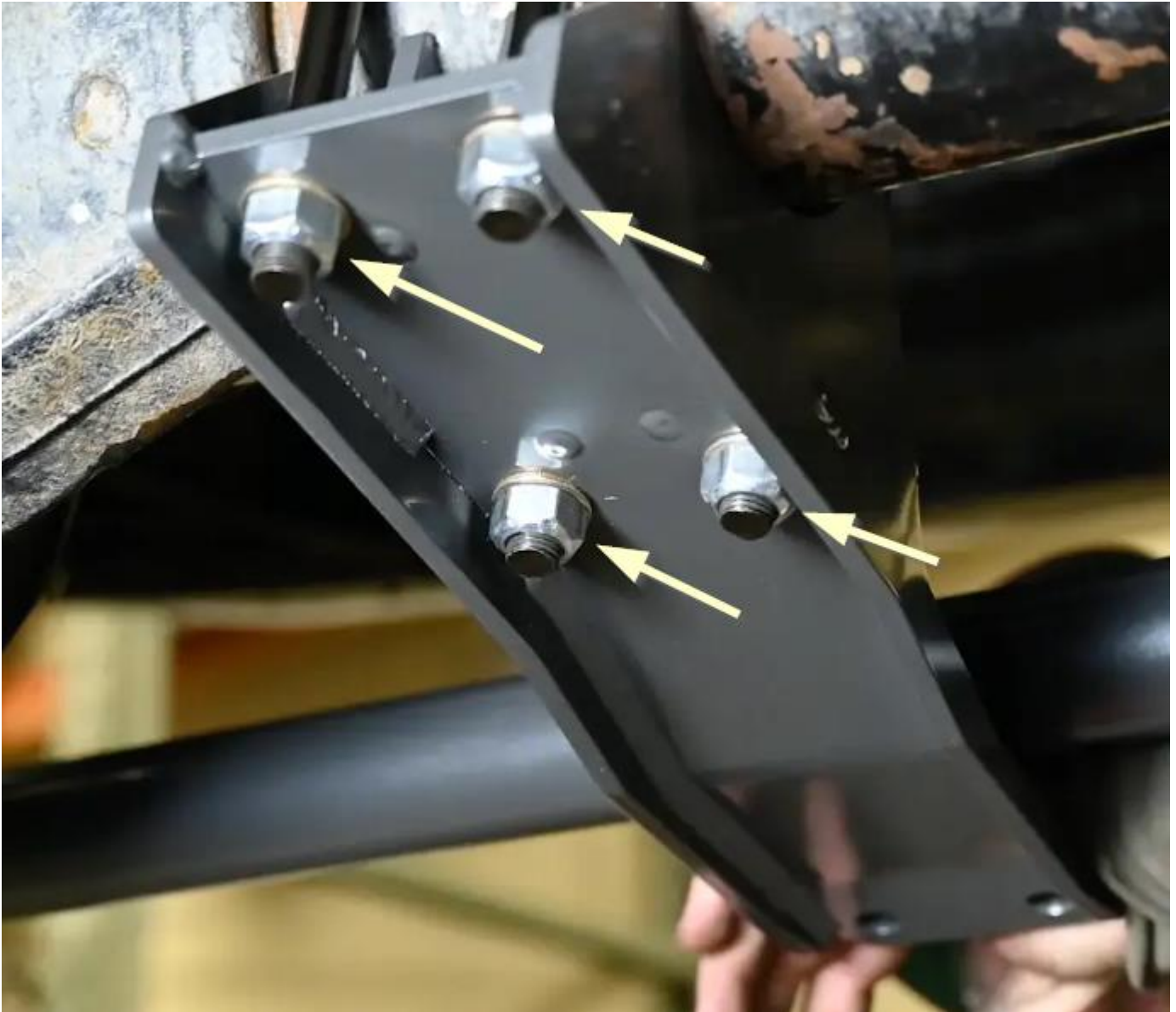
Figure 1. Bolts to Hold the Dual Stabilizer Bracket
