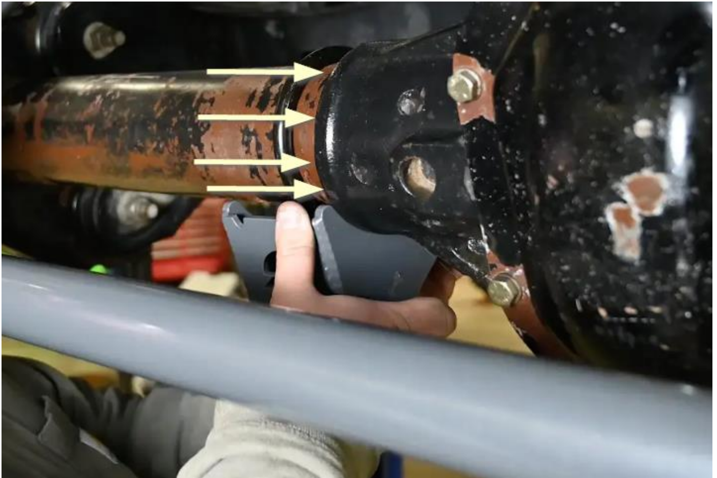
Figure 2. Dual Stabilizer Bracket Indexed on the Differential Housing
