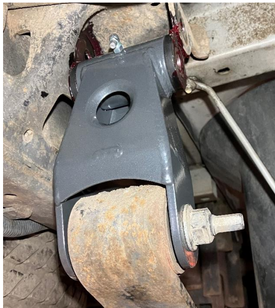
Figure 4. New Shackle Loosely Bolted to the Leaf Spring Eyelet.
