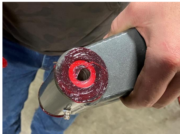
Figure 2. Greased Bushing Faces on New Shackles.
