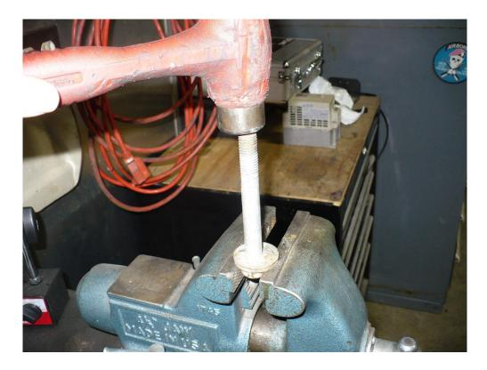
4. With bolt removed, install the new stepped cam bolt eliminators. Dimensionally, the stepped cam bolt eliminators are the same, there is not one press fit and one slip fit like the OEM design. Install the stepped cam bolt eliminators onto the vehicle, with the raised end of the eliminator sitting inside the factory slot on the control arm bracket. See image below for proper installation.
