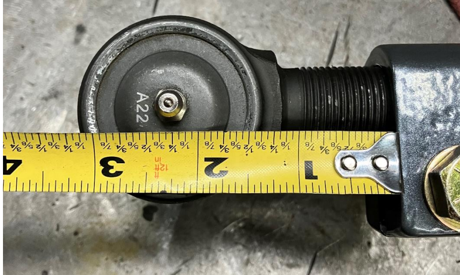
Figure 9. Passenger Side TRE Adjusted to 2 1/4" From End of Tie Rod Forging.
