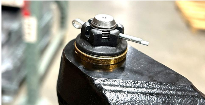
Figure 6. Washer Installed to Engage Cotter Pin and Castle Nuts Slots
