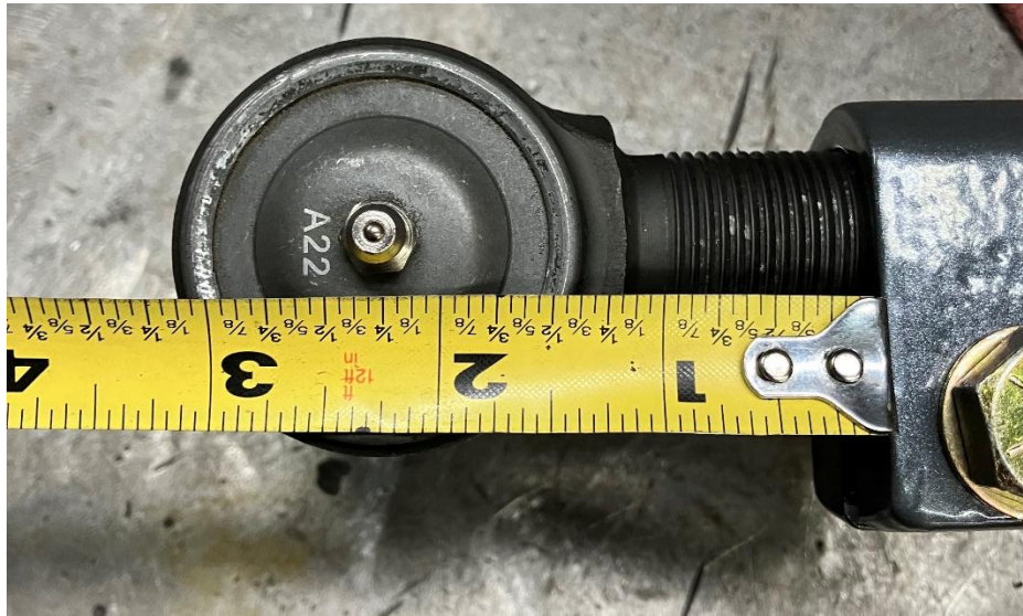
Figure 2. Passenger side TRE adjusted to 2 1/4" from end of tie rod.
