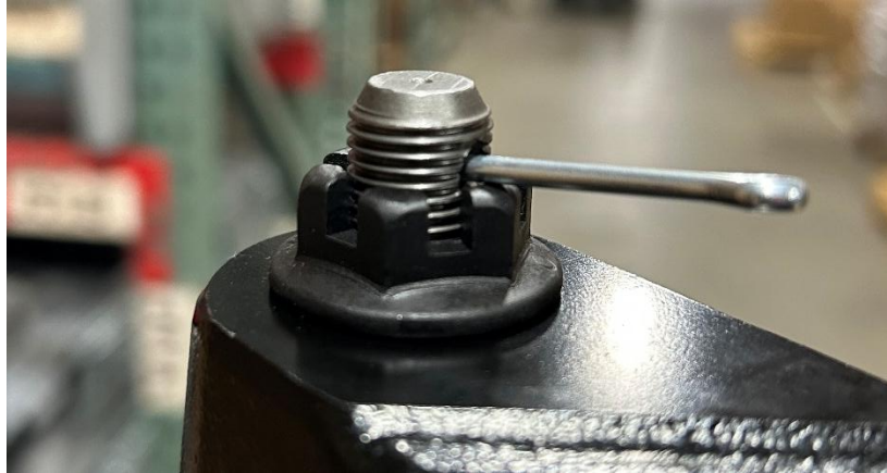
Figure 5. Cotter Pin Not Engaged in Castle Nut Slots
