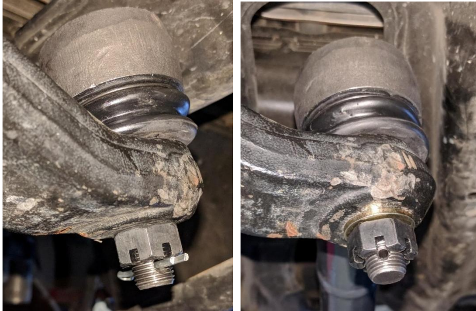
Figure 14 and 15. Washer Used Under Castle Nut
