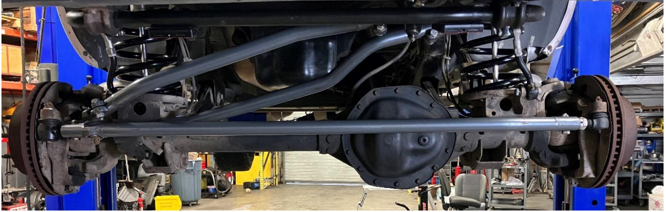
Figure 12. Installed Tie Rod and Drag Link
