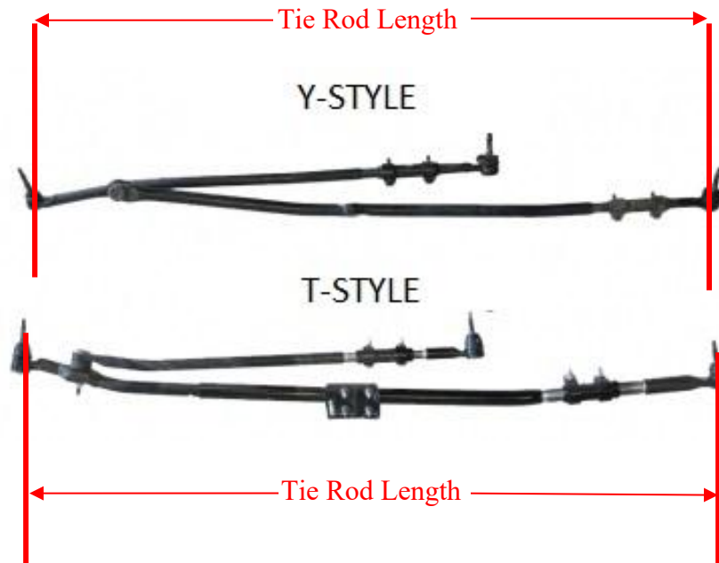
Figure 1. How to Measure Tie Rod Length
