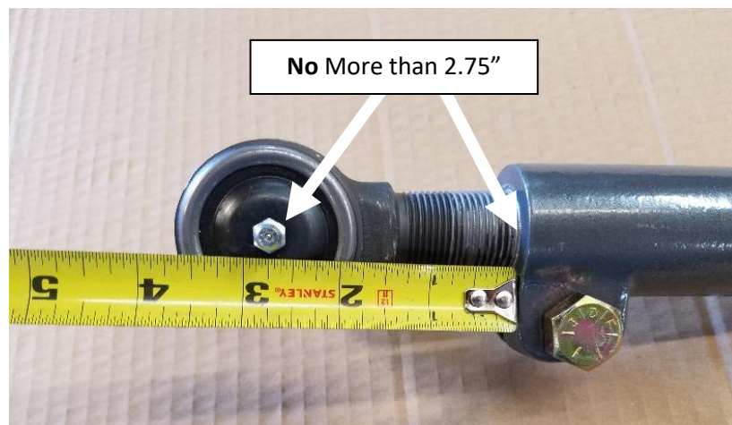
Figure 8. Tie Rod End Adjusted MAX 2.75" Out (Non-Double Adjuster Side)
