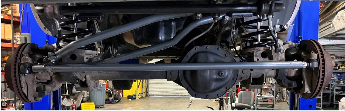
Figure 12. Installed Tie Rod and Drag Link
