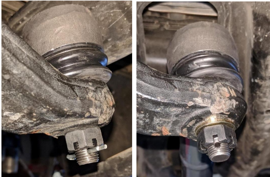
Figure 15 and 16. Washer Used Under Castle Nut
