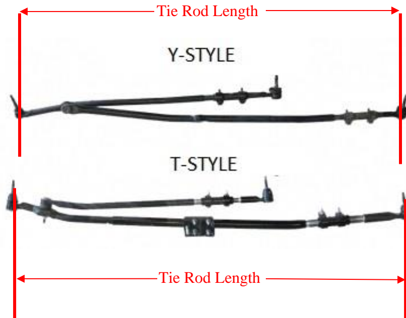
Figure 1. How to Measure Tie Rod Length
