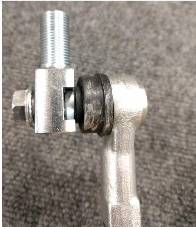
Figure 3. Properly Assembled Sway Bar End Link
