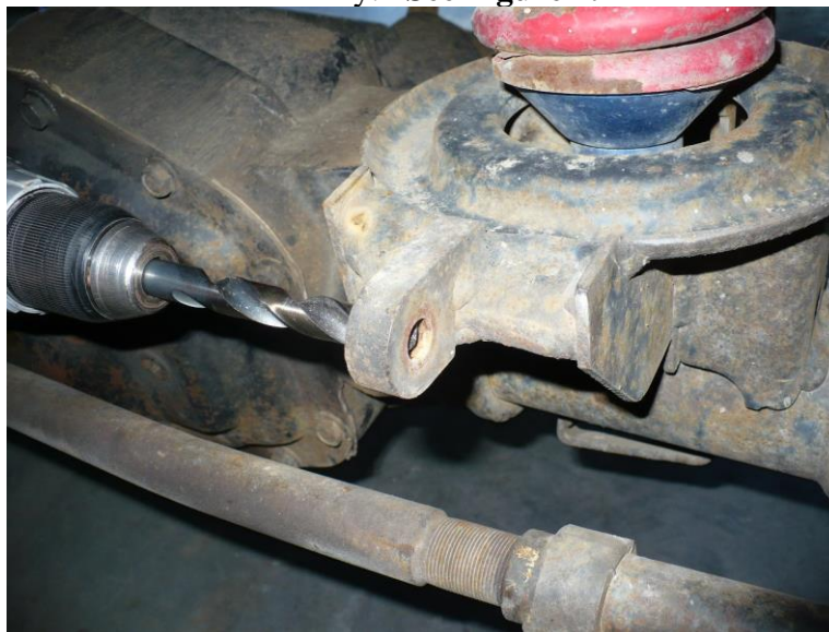
Figure 2. Drilling Out Lower Mount to 1/2"
