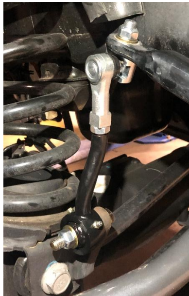
Figure 4. Correctly Installed Sway Bar End Link (2014+)
