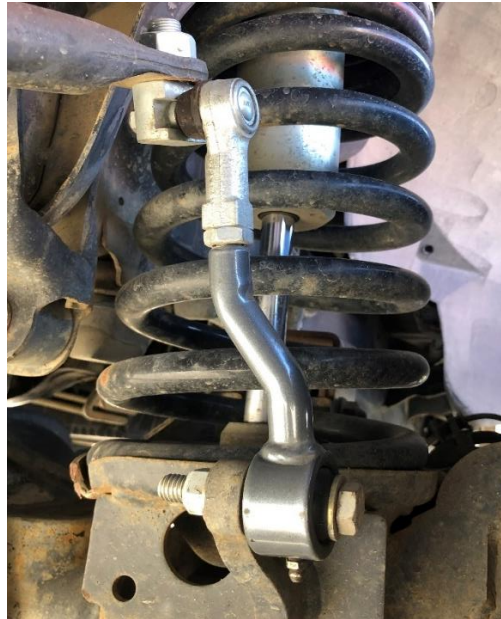
Figure 5. Correctly Installed Sway Bar End Link (2003-2013)
