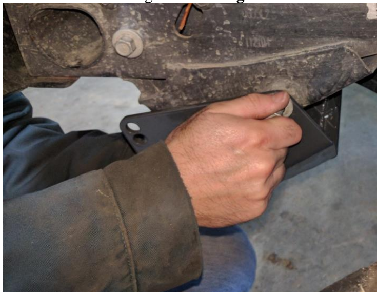
Figure 2. Installing First Bolt in Steering Box Brace
