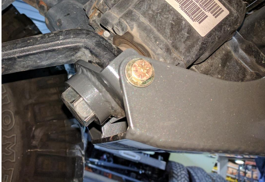
Figure 5. Sector Shaft Brace Installed
