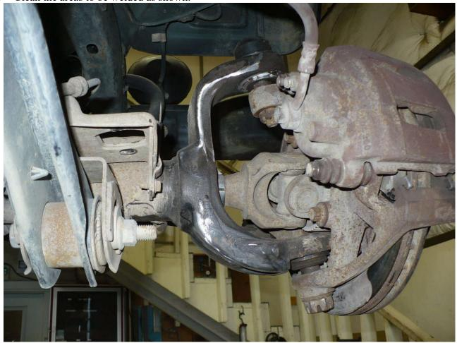
5) Once weld surfaces are prepared, place upper C-gussets in position. There will likely be a slight gap around the ball-joint area; use a C-clamp or vice grips to tighten the gusset in the proper welding
