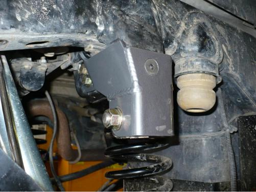
9) Reinstall rear tire and lower vehicle to the ground. Connect track bar and new track bar bolt and torque to 125 lb-ft with the vehicle at ride height.
