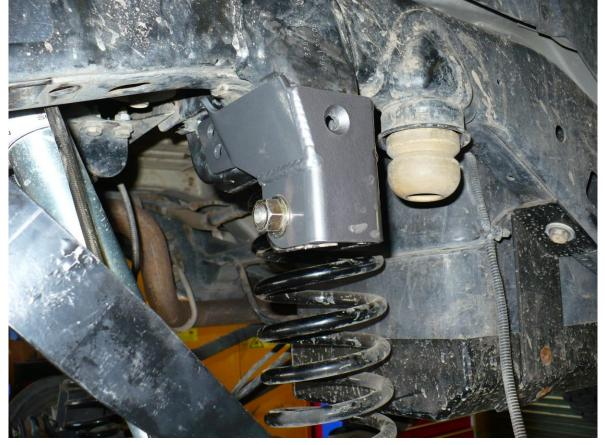
4) Start the 2 7/16" bolts and 1/2" bolt as shown in the pictures below. Do not tighten yet. Simply start bolts and nuts to align bracket.
