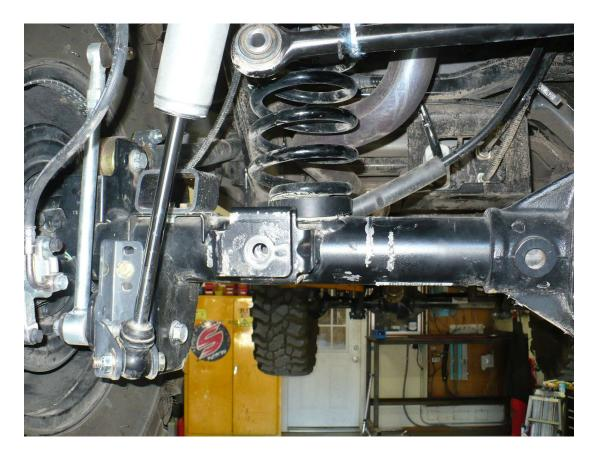
2) Next, slide the bracket over the factory track bar bracket. The new 8076 bracket should sandwich the factory bracket as shown in the pictures below.
