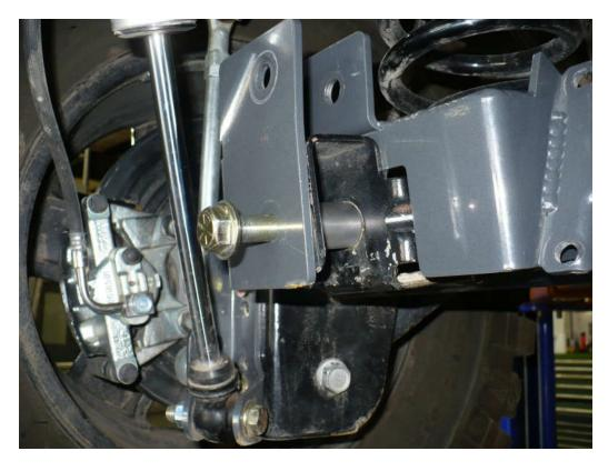
6) Next, install the washer and nut on the back side of the bracket. Do not tighten at this time though.
