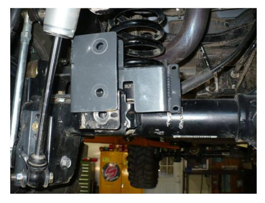
3) At this point, a gentle tap to the top of the bracket with a rubber mallet will seat it into place.
