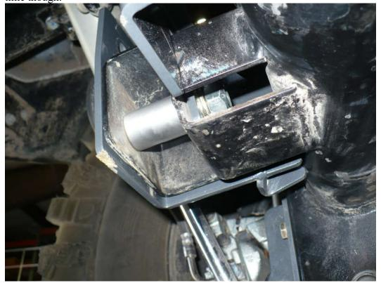
7) Next, install the u-bolts over the axle tube through the track bar relocation bracket. Use a flat washer and nylock nut to secure the u-bolts. On some rear axle housings there is a weld along the front of the axle tube opposite of the track bar bracket. Grind the weld down just where it goes under the u-bolt so that the u-bolt contacts the entire tube.
