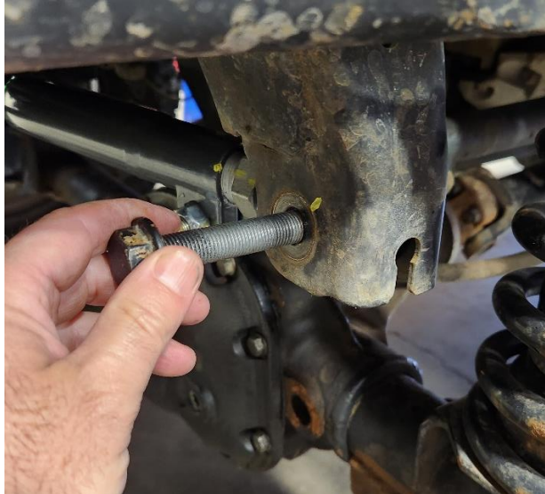
Figure 1. Removing Frame Side Track Bar Bolt
