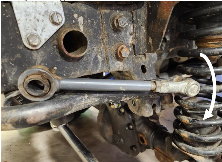
Figure 2. Sway Bar Disconnected and Can Now Be Rotated Down
