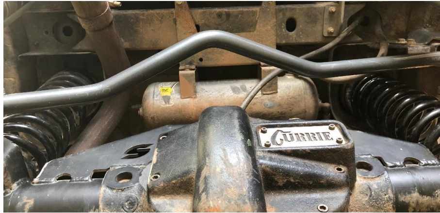
Figure 5. Correct Bend Orientation of Synergy Mfg JK Rear Track Bar
