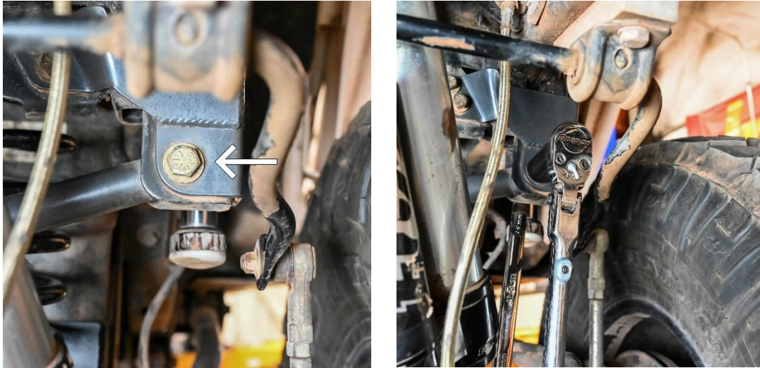
Figures 2 and 3. Removing the Track Bar from the Frame Side
