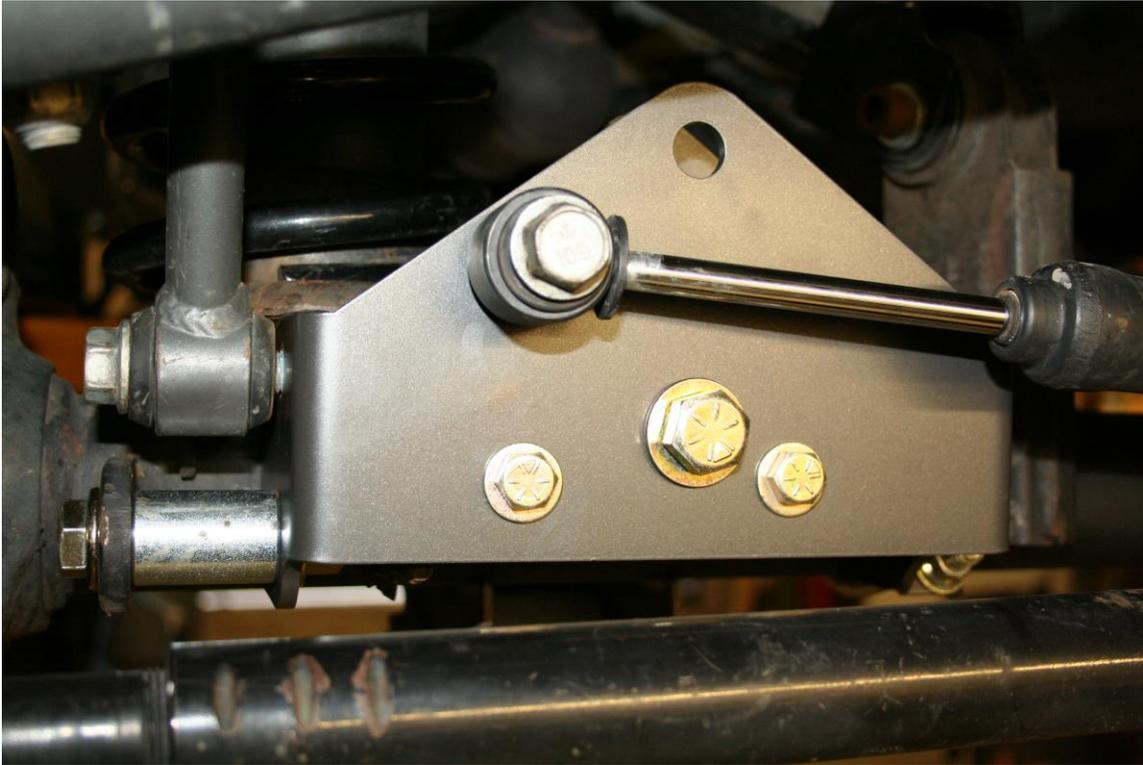
13. Reattach the track bar using the factory nut and bolt, it helps to have someone turn the steering wheel to align the track bar to the hole in the bracket.
