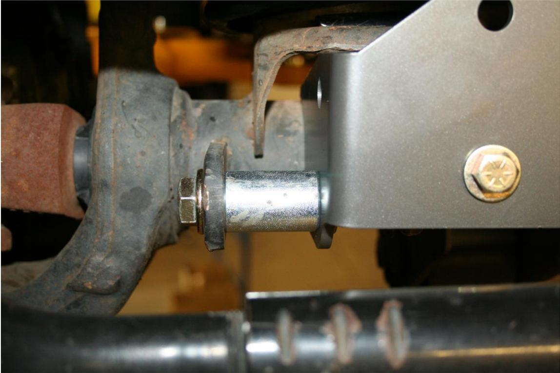
8. Install the driver side anti-sway bar relocation bracket using a 1.5" spacer and  $\frac{1}{2}$ " x 3" bolt and top-lock nut; use a washer under the bolt-head and nut.
