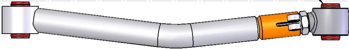
5. Install the new control arms with the adjuster at the frame end. The arms are bent in for tire clearance, and up for ground clearance. Be sure to install them correctly. Reuse the factory mounting bolts.
