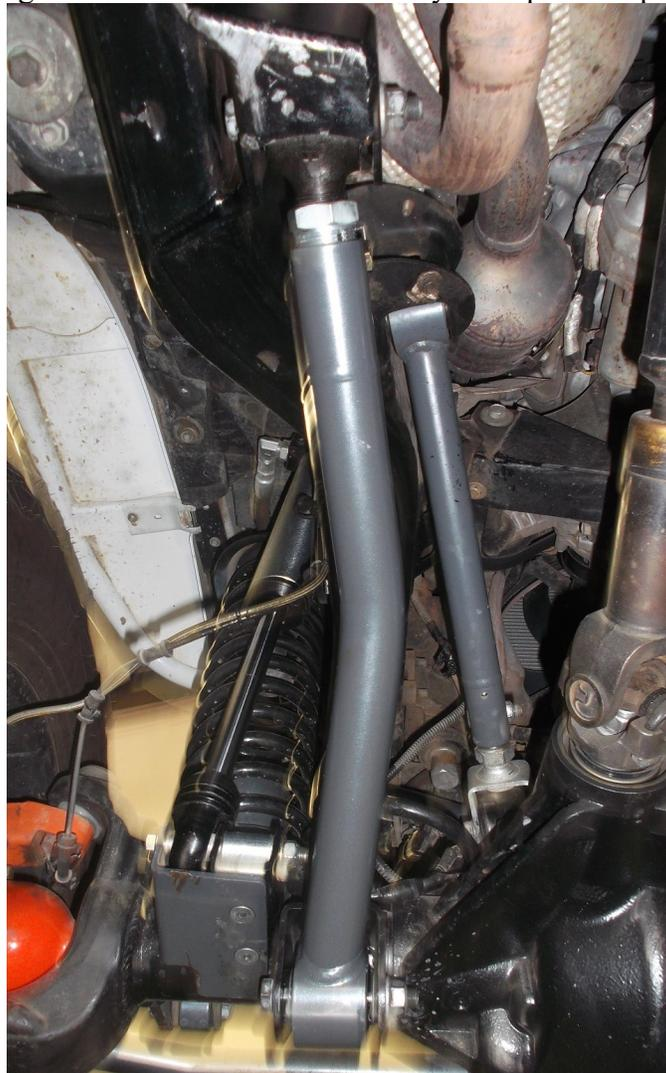
6. Tighten the factory control arm bolts to 125 ft-lbs. Once final length adjustments are made, ensure the vehicle is at ride height and tighten the pinch bolt to 80 ft-lbs. Put a wrench on the adjuster sleeve at this time and try to move the adjuster. Make sure pinch bolt has adequately clamped onto the flex joint shank so that the adjuster is not movable. If movable, increase torque on pinch bolt but do not exceed 90 ft-lbs.
