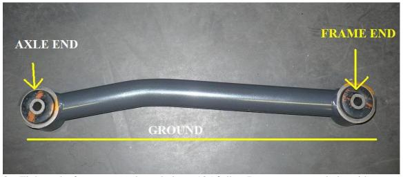
3. Tighten the factory control arm bolts to 125 ft-lbs. Be sure to torque bolts with vehicle's weight on the suspension as to not preload the control arm bushings.
