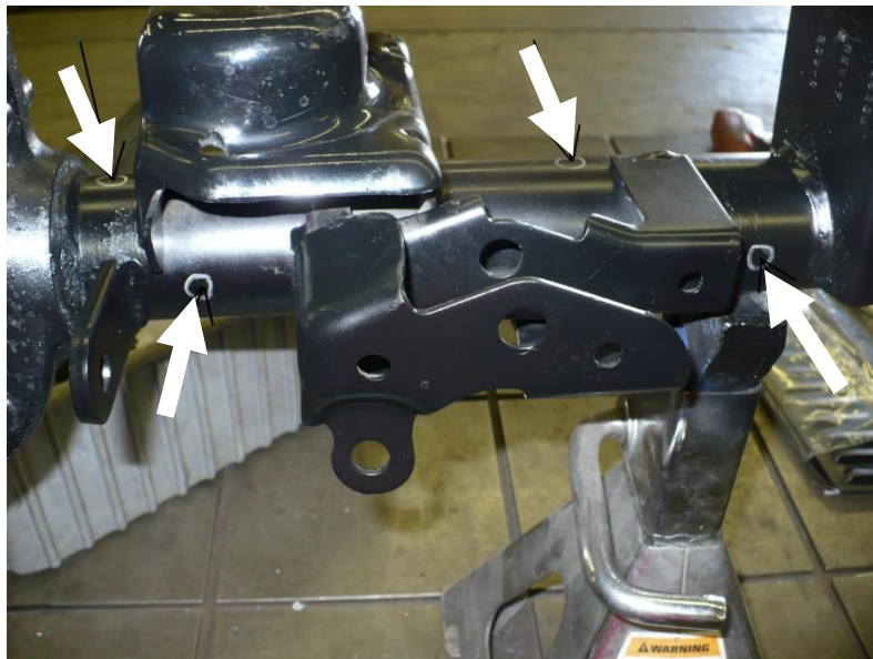
Figure 3. Marking Hole Locations Outside UCA Bracket On Long Side
