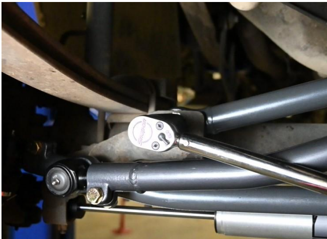
Figure 5. Torquing Axle Side Bolt
