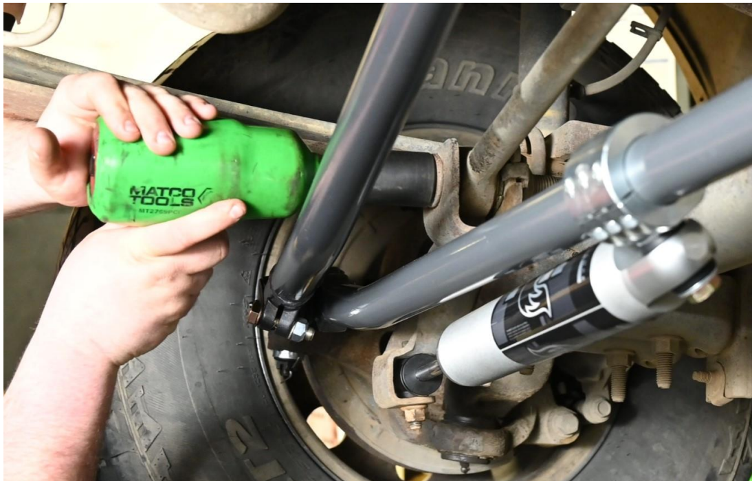
Figure 1. Unbolting the Axle Side of the Front Track Bar
