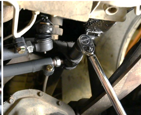
Figure 6. Torquing Frame Side Bolt
