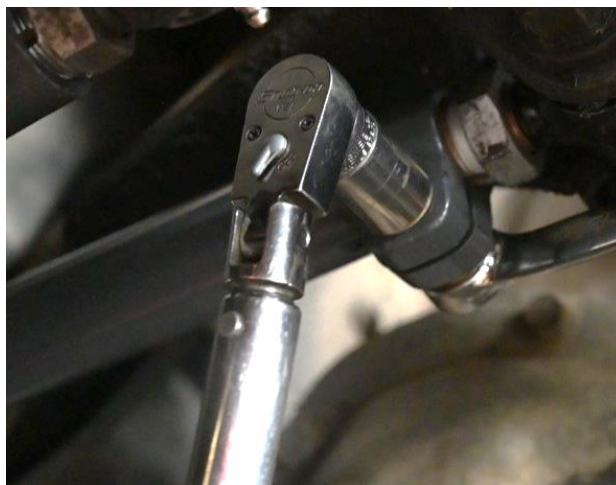
Figure 9. Tightening Pinch Bolt.
