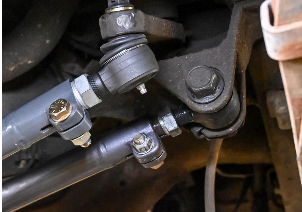
Figure 4. Installing the Frame Side Bolt and Nut
