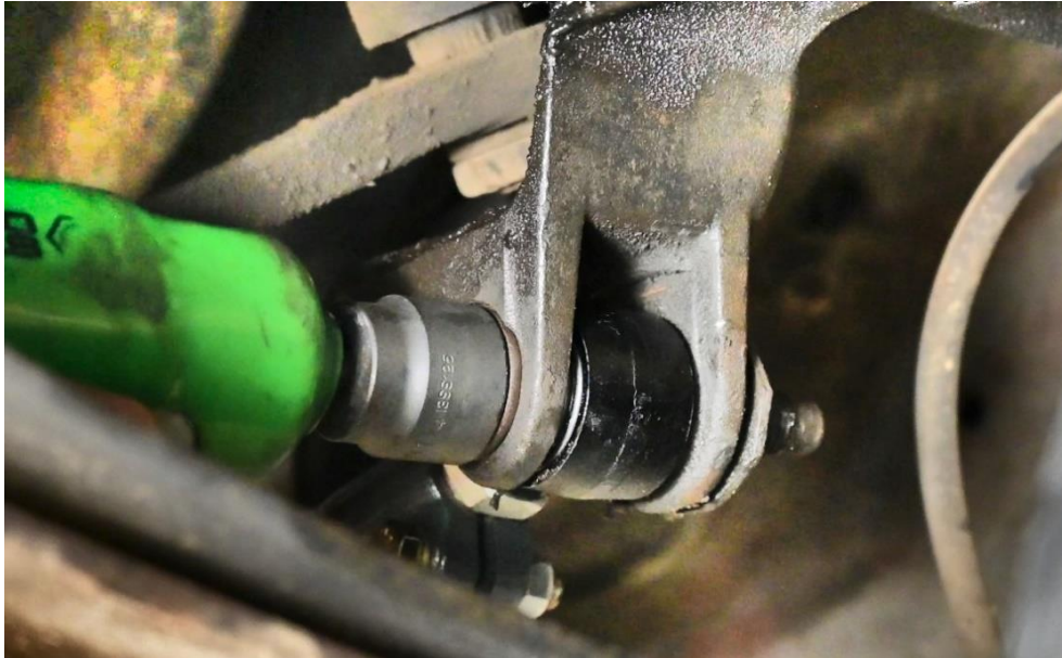
Figure 2. Unbolting the Frame Side of the Front Track Bar
