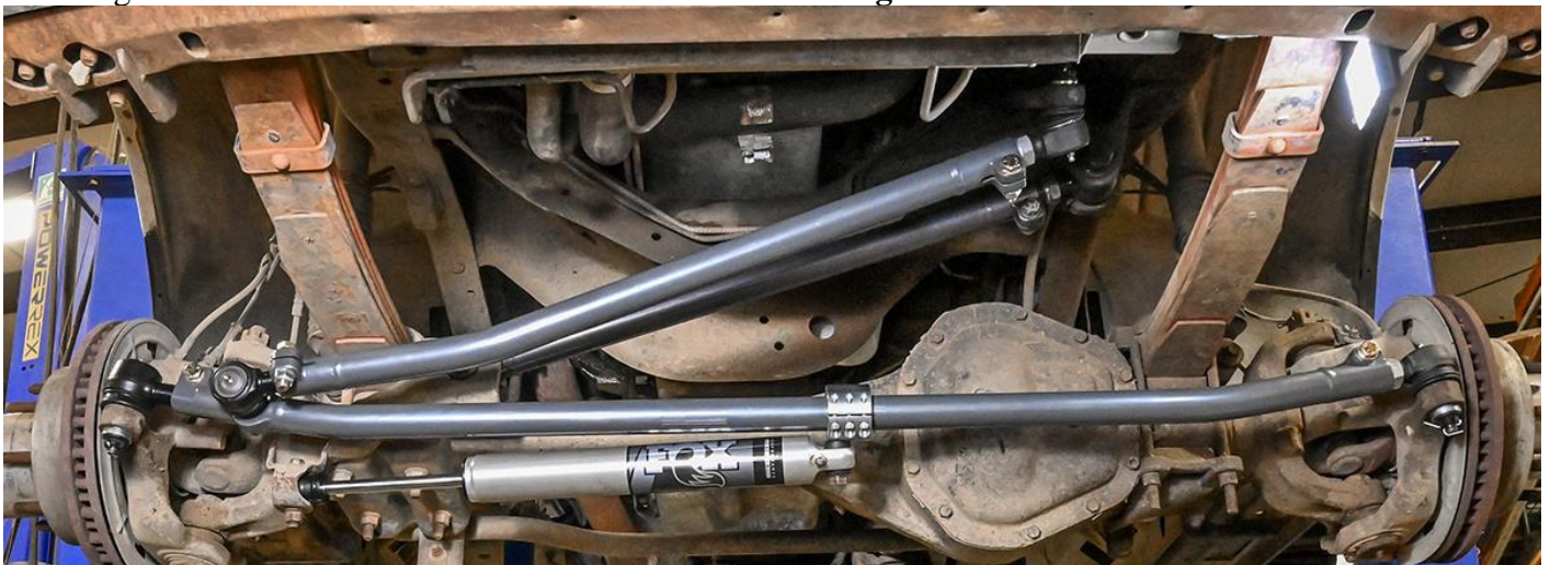
Figure 1. Aligned Tie Rod with Passenger Side Pinch Bolt Tight.
