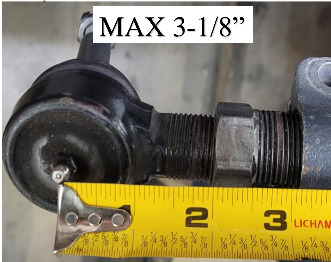
Figure 2. Double Adjuster Tie Rod End Maximum Extension.
