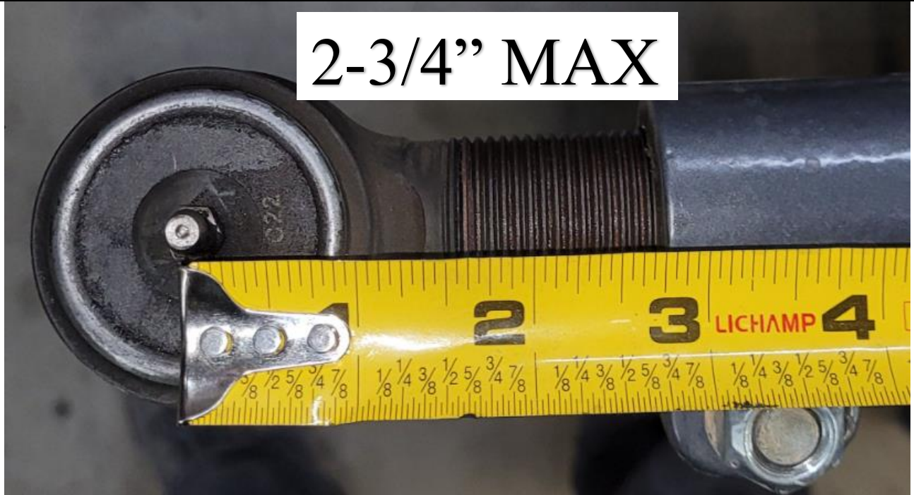
Figure 3. NON-Double Adjuster Tie Rod End Maximum Extension
