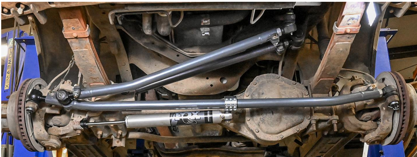
Figure 4. The Synergy Drag Link Installed in the Truck
