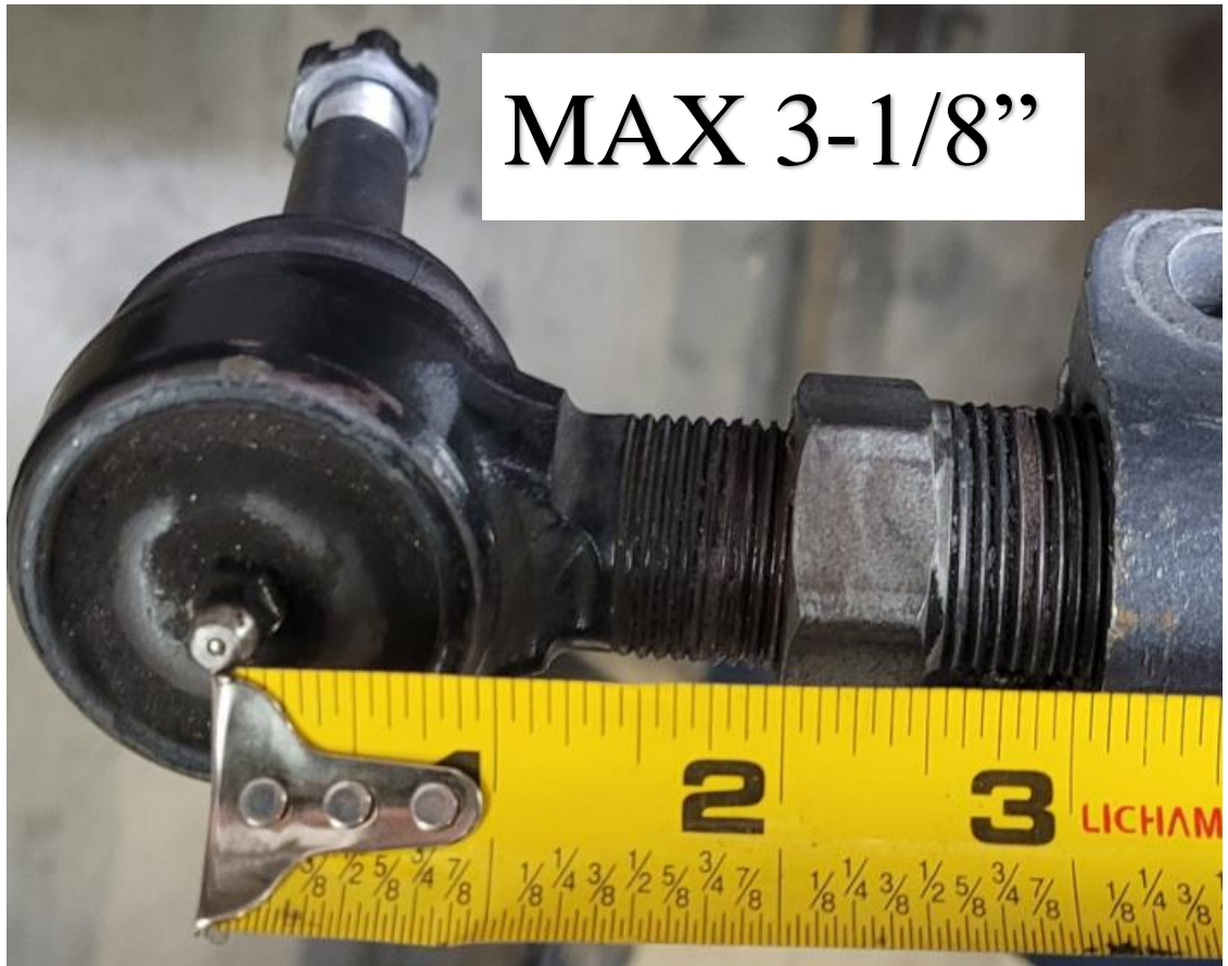
Figure 4. Double Adjuster Rod End Adjusted to MAX 3-1/8”.
