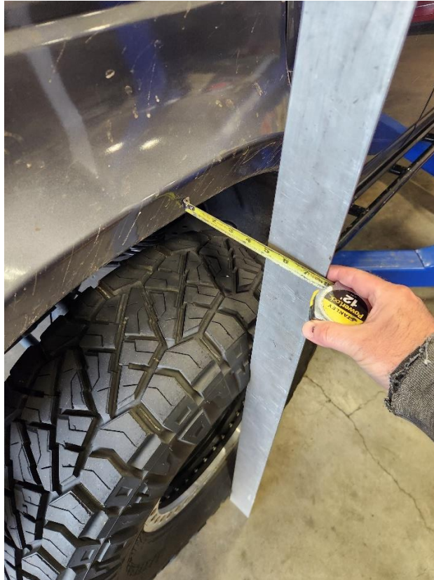
Figure 7. Measuring Side to Side to Center the Body Over the Axle.
