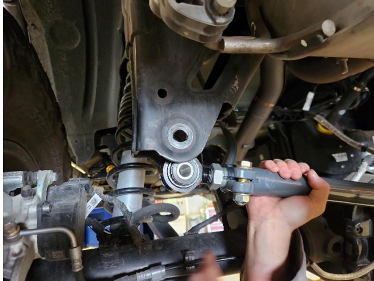
Figure 5. Installing the Synergy Mfg. Track Bar at the Axle
