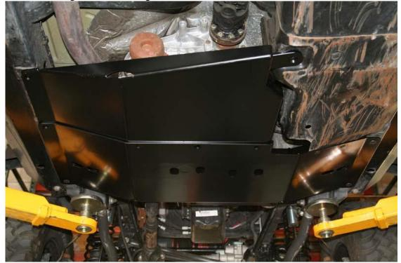
13. Install the 3 center ½" flat head allen bolts with the flange nuts and tighten to 35 ft-lbs.
