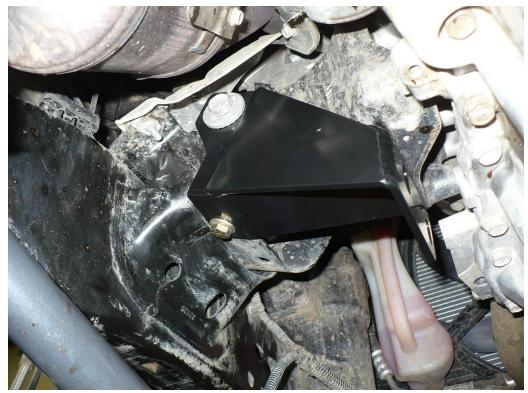
15. Install the driver side frame brace to the frame bracket. The driver side is the shorter of the two.
