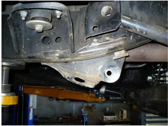
21) Next, carefully cut the inner part of the lower control arm bracket as shown below. Be careful not to cut through the frame.
