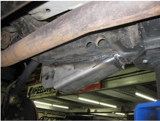
28) Allow welds to cool. Deburr welds and paint to prevent corrosion.
