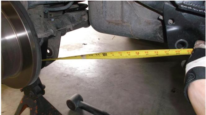
19) With measurements in hand, begin cutting rear lower control arm mount off the vehicle. 20) Begin by cutting the outer half of the bracket off, as shown below. This may take multiple cuts to
