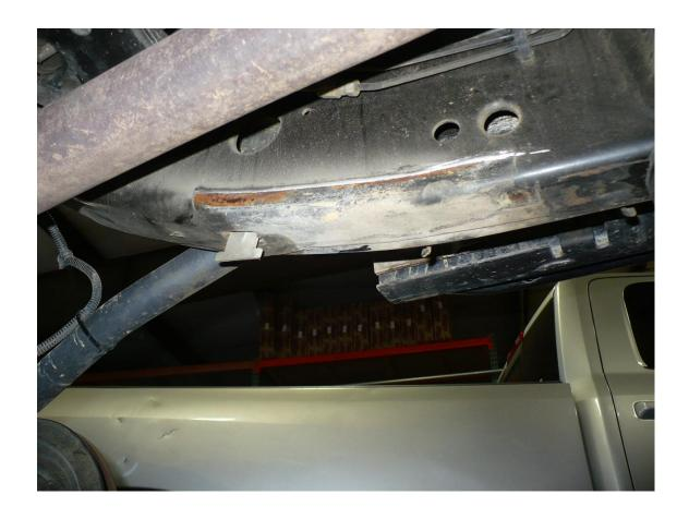
22) With bracket fully removed as shown above, grind smooth the frame.
