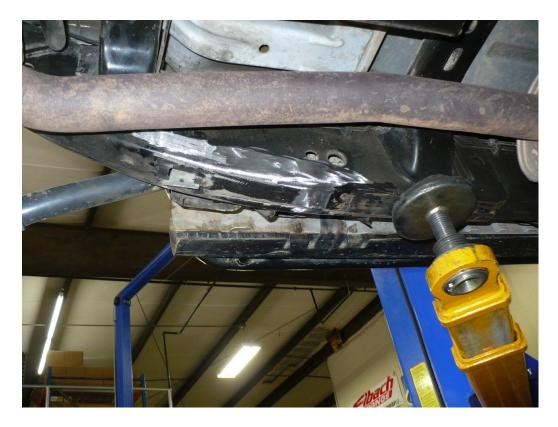
23) Test fit the bracket. The keyway on the bracket was intended to self-locate the bracket off the body mount as shown below. The rear side of the keyway should meet with the rear side of the body mount.
