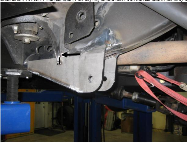
24) Use a clamp to hold the bracket into position and match the measurements taken in step 18.
